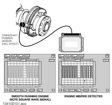
In order to eliminate misfire faults that can occur as a result of varying flywheel tolerances (manufacturing process) an internal adaptation of the flywheel is made. The adaptation is made during periods of decel fuel cut-off in order to avoid any rotational irregularities which the engine can cause during combustion. This adaptation is used to correct segment duration periods prior to evaluation for a misfire event.
