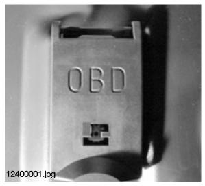
The OBD II connector is located in the driver's footwell to the left of the steering column for E39, E46 and E53 vehicles.
