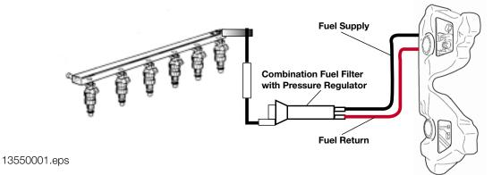
The fuel rail distributes an even supply of fuel to all of the injectors, and also serves as a volume reservoir. The fuel rail is secured by bolts to the intake manifold.
