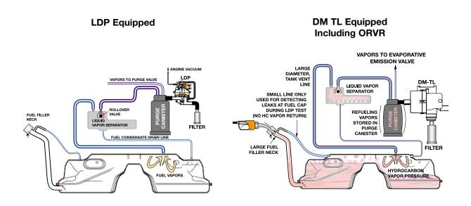
**Evaporative Emissions:** The control of the evaporative fuel vapors (Hydrocarbons) from the fuel tank is important for the overall reduction in vehicle emissions. The evaporative system has been combined with the ventilation of the fuel tank, which allows the tank to breath (equalization). The overall operation provides:
