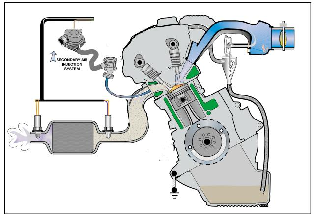
**Exhaust Emissions:** The combustion process of a gasoline powered engine produces Carbon Monoxide (CO), Hydrocarbons (HC) and Oxides of Nitrogen (NOx).
