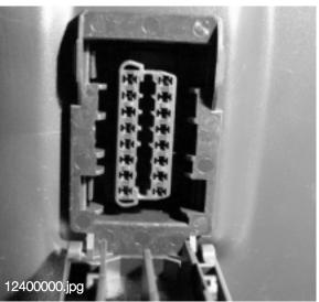
The cap to the OBD II connector contains a bridge that links KL 30 to TXD and TXD II. This is to protect the diagnostic circuit integrity and prevent erroneous faults from being logged.
