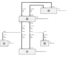
The data required for engine torque manipulation is relayed via the CAN bus.
