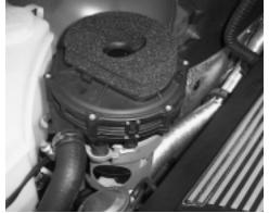
The Air Injection Inlet Valve mounts directly to the cylinder head, with a passageway machined through the head. This eliminates the external Air Injection manifold distribution pipes to the exhaust manifolds.
