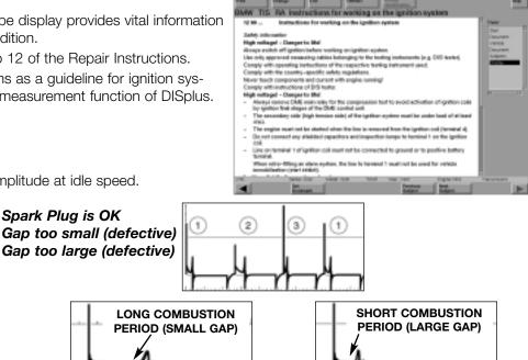
Evaluation of secondary signal amplitude at idle speed.
