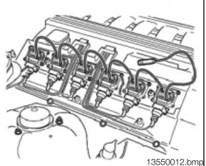
The Spark Plugs should be properly installed and torqued using the following Special Tools:
