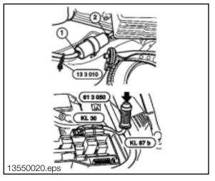
When testing fuel pressure, the hand held fuel pressure gage (#13 3 060) can be used.
