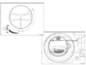
Please check the fuel filler cap first when the dashboard light comes on to avoid unnecessary diagnostic time. To check the fuel filler cap turn the cap to the right until you hear a click or the cap reaches the full stop. Make sure that the retaining strap is not caught between the filler pipe and the fuel filler cap. If the light should stay on further in depth evaporative leak diagnosis is required.
