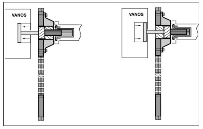
The operation of the VANOS solenoid is monitored in accordance with the OBD II requirements for emission control. The ECM monitors the final stage output control and the signal from the Camshaft Position Sensors for VANOS operation. Dual VANOS consists of the following parts:
