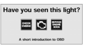
This light informs the driver of the need for service, NOT of the need to stop the vehicle. A blinking or flashing dashboard light indicates a rather severe level of engine misfire.
