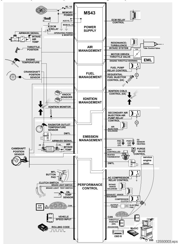
System Components: Inputs - Processing - Outputs
