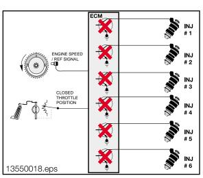
When the engine rpm approaches idle speed, the injection ms value is increased (cut-in) to prevent the engine from stalling. The cut-in rpm is dependent upon the engine temperature and the rate of deceleration. This function can be observed as displayed on the Fuel Economy (MPG) gauge.
