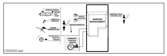
The ECM has a very "broad" range of ignition timing. This is possible by using a Direct Ignition System, or sometimes refered to as "Static Ignition System" (RZV). Reliability is also increased by having separate individual ignition circuits.
