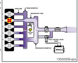
When the engine speed is greater than 3750 RPM the solenoid is de-energized. The resonance flap is sprung open, allowing flow through both resonance tubes, increasing volume.
