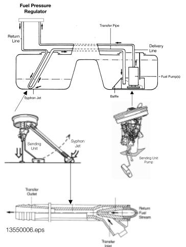
**Fuel Pump:** The electric fuel pump supplies constant fuel volume to the injection system. This system uses a single submersable (in the fuel tank) pump. The inlet is protected by a mesh screen.
