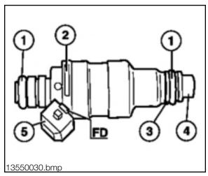
Fuel injectors can leak which bleeds off fuel pressure and increases emissions. The injectors can be tested using the Fuel Injector Leakage Tester.
