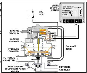
During every engine cold start the LDP solenoid is energized by the ECM. Engine manifold vacuum enters the upper chamber of the LDP to lift up the spring loaded diaphragm.
