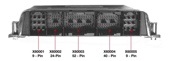
The 134 pin ECM is manufactured by Siemens to BMW specifications. The ECM is the SKE (standard shell construction) housing and uses 5 modular connectors. For testing, use the Universal Adapter Set (break-out box) Special Tool # 90 88 6 121 300.
