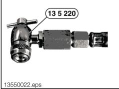
When testing the fuel injectors for leakage, use Special Tool #88 88 5 000 362. Leak testing the fuel injectors is one of the diagnostic steps listed in "Long Cranking Times" S.I. #13 08 90 (3096). This tool pressurizes the injectors with air and the injector tips are submersed in water. If air bubles are present, this indicates the leaking injector(s).
