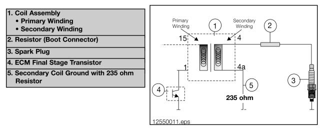
The Coil Assembly contains two copper windings insulated from each other. One winding is the primary winding, formed by a few turns of thick wire. The secondary winding is formed by a great many turns of thin wire.
