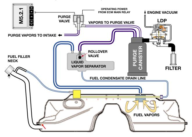
• During diagnostic testing of the evaporative emission system, the vent valve is closed and will block atmospheric venting. The purge valves are also sprung closed to seal the system.
