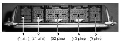
The modular harness connectors are color coded by cylinder bank on the M73. When removing control modules from the E-Box, note the color of the plugs and mark each module to prevent incorrect replacement. This step is important to prevent EWS III (3.3) ISN incompatibility.
