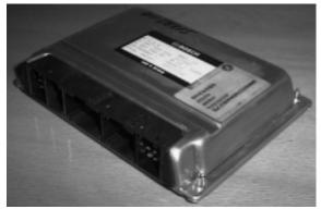
M5.2.1 control modules utilize the **SKE** (standard shell construction housing). The SKE utilizes a modular connector configuration. There are a total of 5 connectors providing a combined total of **134 pins.**
