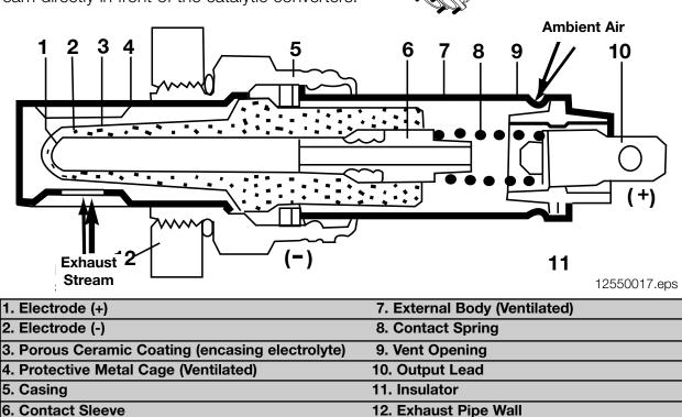
The "tip" of the sensor contains a microporous platinum coating (electrodes) which conduct current. The platinum electrodes are separated by solid electrolyte which conducts oxygen ions. The platinum conductors are covered with a highly porous ceramic coating and the entire tip is encased in a ventilated metal "cage".
