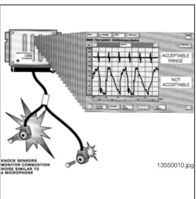
If a fault is detected with the Knock Sensor(s) or circuits, the ECM deactivates Knock Control. The ignition timing will be set to a conservative basic setting (to reduce the risk of detonation) and a fault will be stored. The "Malfunction Indicator Light" will be illuminated when the OBD II criteria is achieved.
