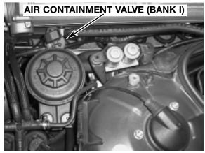
**NOTE:** Air injection will be interrupted during idle at engine operating temperature, if the idle speed becomes too high!
