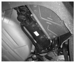
The LDP assembly is only replaceable as a complete unitized component, however, it is separate from the charcoal canister.
