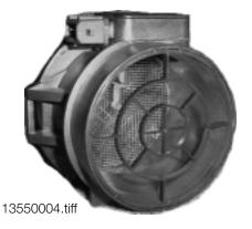
**Air Temperature Signal:** This signal is needed by the ECM to correct the air volume input for changes in the intake air temperature affecting the amount of fuel injected, ignition timing and Secondary Air Injection activation. The sensor is located in the center of the intake manifold (1).
