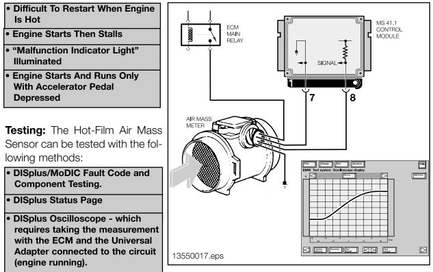
**NOTE:** Visually inspect the sensor for damaged, missing or blocked screens. The screens affect air flow calibration. Also inspect the sealing rings where the sensor inserts in the air filter housing and intake boot. Ensure the pin connections are tight.
