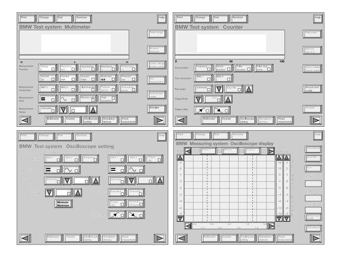
**MEASUREMENT SYSTEM WORKSHEET:** While connecting and setting up the DIS/MoDiC measurement system for signal/circuit validation, note the settings in the appropriate locations for future reference. Document your findings by entering the displayed values in the Multimeter or Counter Display. If the signal requires the use of the oscilloscope, note your set up selections and sketch the waveform.
