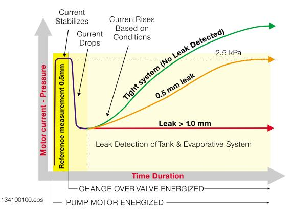
If the ECM detects a leak, a fault will be stored and the "Malfunction Indicator Light" will be illuminated. Depending on the amperage measurement detected by the ECM, the fault code displayed will be "small leak" or "large leak".
