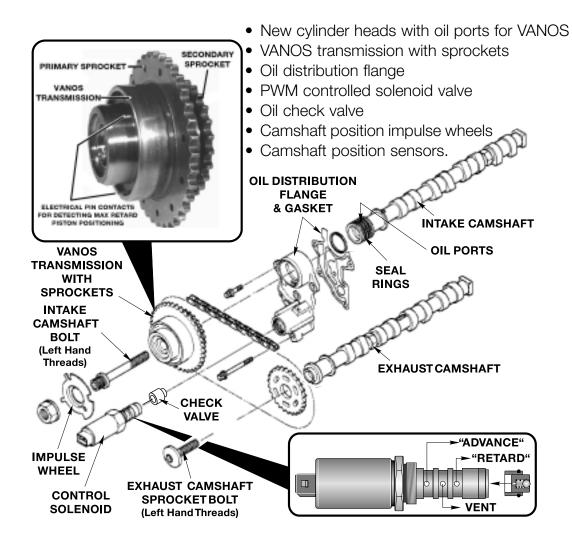
**VANOS CONTROL SOLENOID & CHECK VALVE:** The VANOS solenoid is a two wire, pulse width modulated, oil flow control valve. The valve has four ports;
