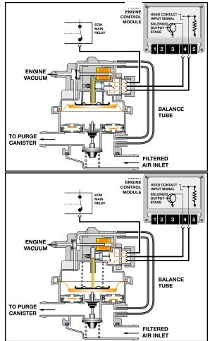
This electrically controlled repetitive up/down stroke is cycled repeatedly building up a total pressure of approximately +25mb in the evaporative system. After sufficient pressure has built up (LDP and its cycling is calibrated to the vehicle), the leak diagnosis begins and lasts about 100 seconds.
