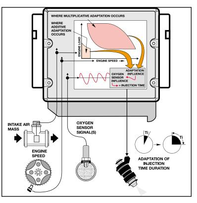
**Adaptation Values** are stored by the ECM iln order to maintain an "ideal" air/fuel ratio. The ECM is capable of adapting to various environmental conditions encountered while the vehicle is in operation (changes in altitude, humidity, ambient temperature, fuel quality, etc.).
