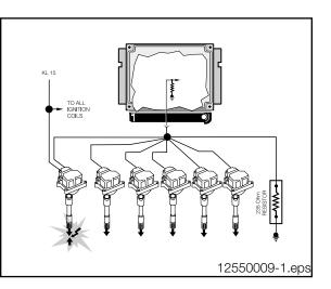
As the secondary magnetic field collapses, a voltage spike is induced in the windings. The ECM monitors the voltage drop across the resistor as an indication of coil firing. After the ECM activates the primary ignition, this feedback signal **(Terminal 4a Signal)** is confirmation that secondary ignition took place. The ECM measures the duration of time it takes the voltage drop for each ignition coil to dissipate below two volts. The time scale constantly changes based on engine rpm.
