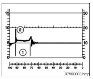
Evaluation of Ignition Voltage Peaks at Idle Speed (Multiple Cylinders Displayed).
