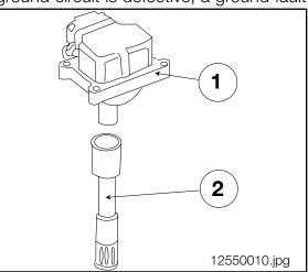
**Spark Plugs:** The spark plugs introduce the ignition energy into the combustion chamber. The high voltage "arcs" across the air gap in the spark plug from the positive electrode to the negative electrode. This creates a spark which ignites the combustable air/fuel mixture.
