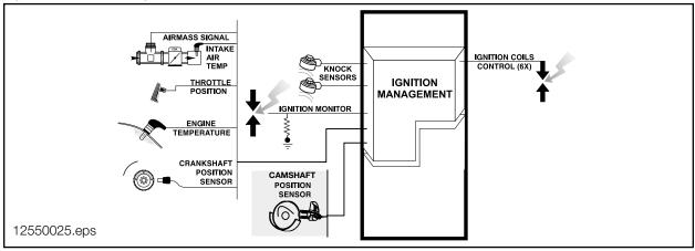
**Ignition Coils:** The high voltage supply required to ignite the mixture in the combustion chambers is determined by the stored energy in the ignition coils. The stored energy contributes to the ignition duration, ignition current and rate of high voltage increase. The Coil circuit including primary and secondary components consists of:
