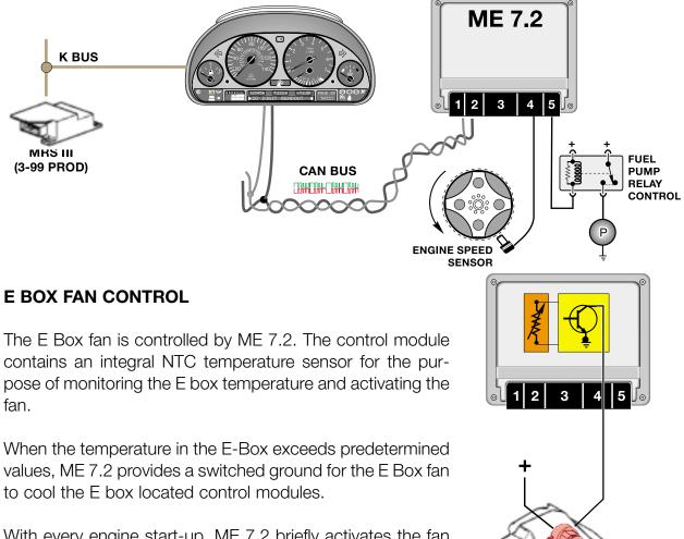
With every engine start-up, ME 7.2 briefly activates the fan ensuring continued fan motor operation for the service life of the vehicle. This feature is intended to prevent fan motor "lock up" from lack of use due to pitting or corrosion over time.
