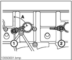
**Crankshaft Position/RPM Sensor:** This sensor provides the crankshaft position and engine speed (RPM) signal to the ECM for ignition activation and correct timing. This input is also monitored for Misfire Detection. For details about the sensor, refer to the Fuel Management section.
