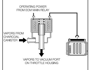
The Evaporative Emission Valve is opened in stages to moderate the purging.
