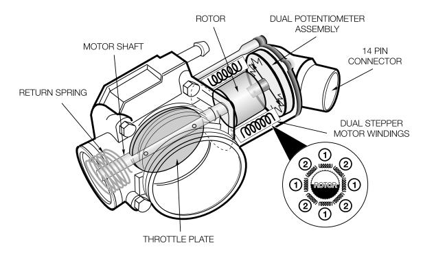
The dual feedback potentiometers signal the movement and position of the throttle plate to each processor. The two potentiometers have separate power and ground circuits to ensure the reliability of their operation.
