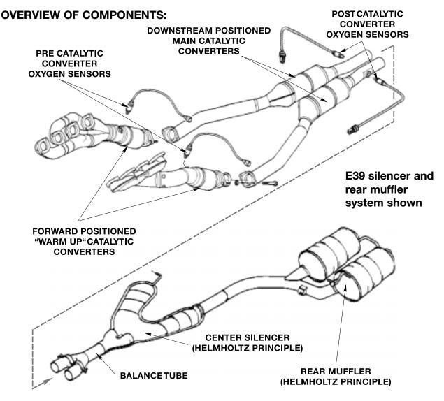
The forward mounted warm-up catalytic converters are made of thin-wall ceramics. They are mounted in a pliable material called silicatex which isolates them from vibrations ensuring a long service life.
