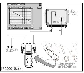
If the Coolant Temperature Sensor input is faulty, a fault code will be set the ECM will assume a substitute value (80° C) to maintain engine operation.
