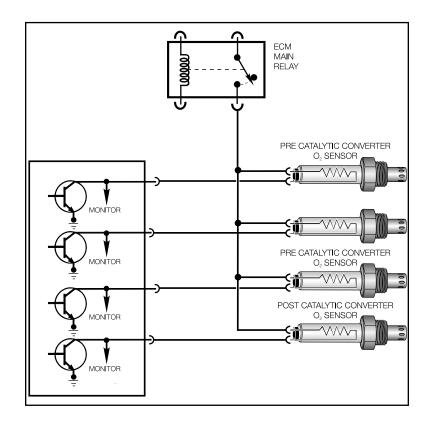
**Catalytic Converter Monitoring:** The efficiency of catalyst operation is determined by evaluating the oxygen consumption of the catalytic converters using the pre and post oxygen sensor signals. A properly operating catalyst consumes most of the O2 (oxygen) that is present in the exhaust gas (input to catalyst). The gases that flow into the catalyst are converted from CO, HC and NOx to CO2, H2O and N2 respectively.
