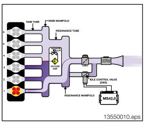
This creates a "block" for the in rushing air. The air flow will stop and expand back (resonance wave back pulse) with the in rushing air to cylinder #5.
