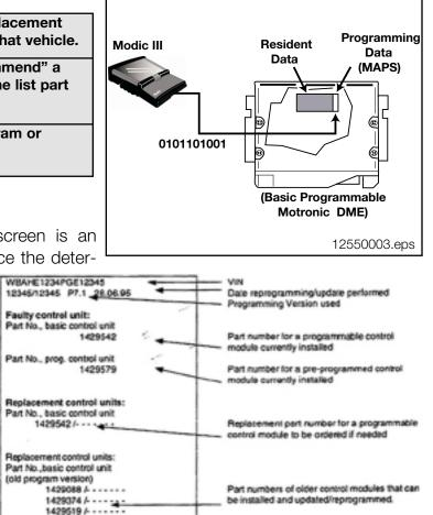
The determination identification screen is an example of the data displayed once the determination is made.
