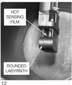
An additional improvement of the HFM 5 is that the hot film element is not openly suspended in the center bore of the sensor as with previous HFMs. It is shrouded by a round fronted plastic labyrinth which isolates it from intake air charge pulsations.
