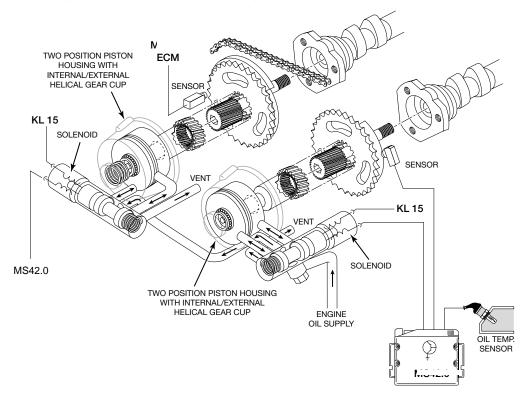
When the engine is started, the camshafts are in the "failsafe" position (deactivated). The intake camshaft is in the RETARDED position - held by oil pressure from the sprung open solenoid. The exhaust camshaft is in the ADVANCED position - held by a preload spring in the actuator and oil pressure from the sprung open solenoid.
