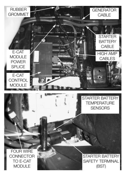
Once the E-CATs are activated, the control module simultaneously provides the output control signal to the dual battery isolation switch (signal KATON) requesting the switch which opens the circuit between the starter battery and vehicle circuit battery. This ensures the E-Cat's operating power is supplied only from the starter battery (detailed description of two battery system further on).
