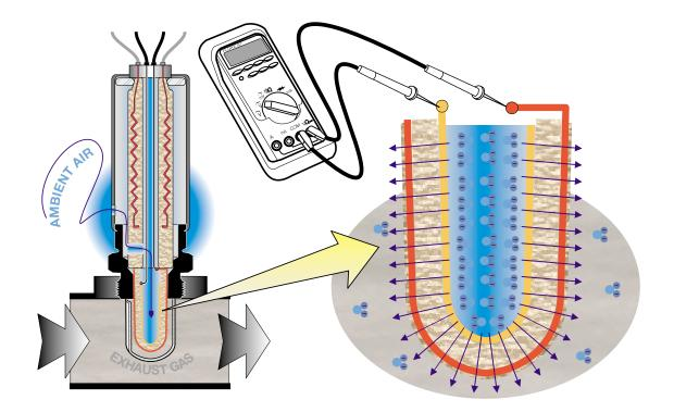
If the exhaust has a lower oxygen content (rich mixture), there will be a large ion "migration" through the sensor generating a higher voltage (950 mV).
