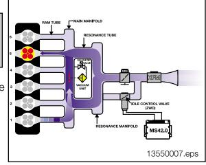
The resonance "wave", along with the intake volume, enhances cylinder filling.
