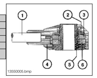
A piezo-ceramic ring is clamped between a seismic mass and the sensor body. When the seismic mass senses vibration (flexing), it exerts a force on the peizo-ceramic element. Opposed electrical charges build up on the upper and lower ceramic surfaces which generates a voltage signal. The acoustic vibrations are converted into electrical signals. These low voltage signals are transmitted to the ECM for processing.
