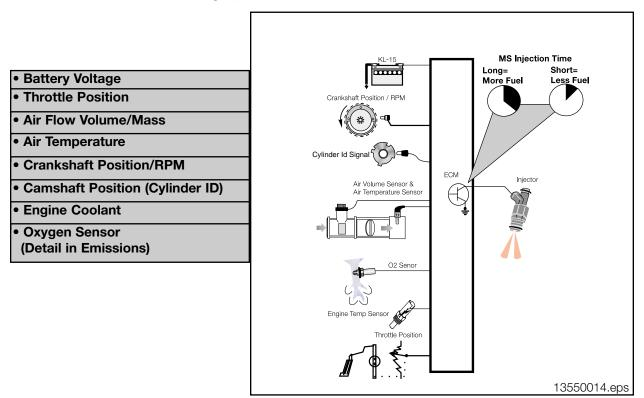
The injection ms value will be regulated based on battery voltage. When cranking, the voltage is low and the ECM will increase the ms value to compensate for injector "lag time". When the engine is running and the battery voltage is higher, the ECM will decrease the injection ms value due to faster injector reaction time.
