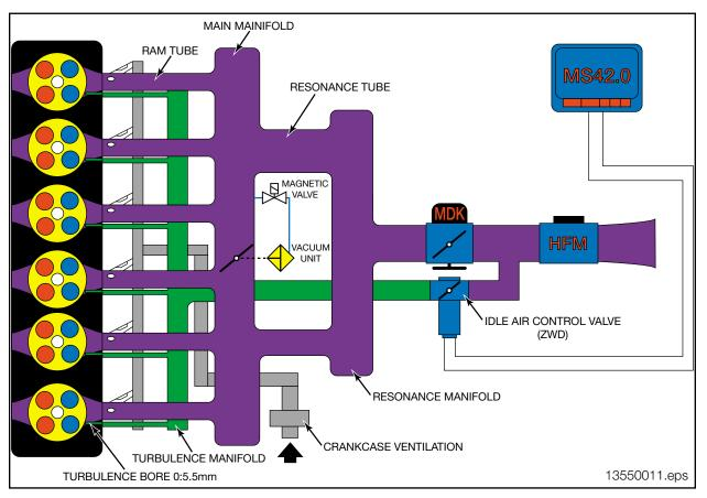
**Resonance System:** The resonance system provides increased engine torque at low RPM, as well as additional power at high RPM. Both of these features are obtained by using an ECM controlled resonance flap (in the intake manifold).
