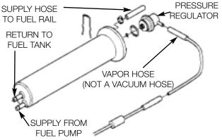
The system provides even fuel distribution to all fuel injectors due to a balance tube connecting the feed with the end of the fuel rail. The new fuel rail does not have a fuel return line.
