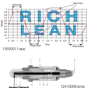
**Direct Oxygen Sensor Heating:** The oxygen sensor conductivity is efficient when it is hot (600° - 700° C). For this reason, the sensors contain heating elements. These "heated" sensors reduce warm up time, and retain the heat during low engine speed when the exhaust temperature is cooler. OBD II requires monitoring of the oxygen sensor heating function and heating elements for operation.
