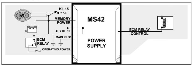
KL30 - Battery Voltage: B+ is the main supply of operating voltage to the ECM.
