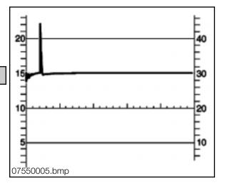
Evaluation of Ignition Voltage Peaks under Sudden Loads (Multiple Cylinders Displayed).
