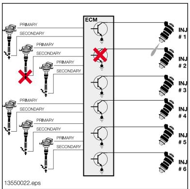
**Fuel Injection Control Monitoring** is performed by the ECM for OBD II requirements. Faults with the fuel injectors and/or control circuits will be stored in memory. This monitoring includes:
