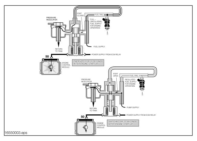
**MS43 Fuel Supply:** The fuel is supplied through a Non Return Fuel Rail System. This system meets Running Loss compliance without the use of the 3/2 Way Valve.
