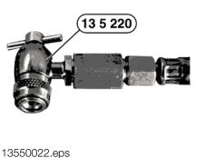
When testing the fuel injectors for leakage, use Special Tool #88 88 5 000 362. Leak testing the fuel injectors is one of the diagnostic steps listed in "Long Cranking Times" S.I. #13 08 90 (3096). This tool pressurizes the injectors with air and the injector tips are submersed in water. If air bubles are present, this indicates the leaking injector(s).
