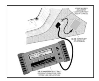
Drive the car in such a manner that all tests listed above can be completed (refer to the drive cycle). When the complete "readiness code" equals "1" (ready) then all tests have been completed and the system has established its "readiness".
