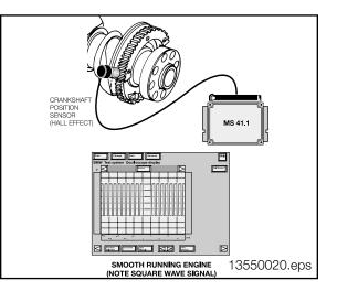
The crankshaft position sensor is monitored as part of OBD II requirements for Misfire Detection. If this input is faulty, the ECM will operate the engine (limited driveability) from the Camshaft Sensor input. A fault with this input will produce the following complaints:
