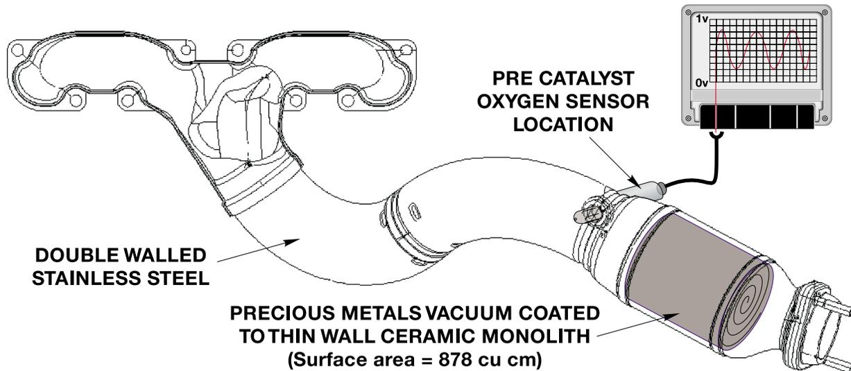
The Bosch LSH 25 oxygen sensors are carried over from the M62 engine and provide the familiar “swinging” voltage signal (0.2 - max lean to 0.8 - max rich) representing oxygen content in the exhaust gas.
