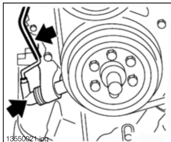
**Camshaft Position Sensor (Cylinder Identification):** The cylinder ID sensor (inductive pulse) input allows the ECM to determine camshaft position in relation to crankshaft position. It is used by the ECM to establish the firing order for the direct ignition system and the semi-sequential fuel injection timing.
