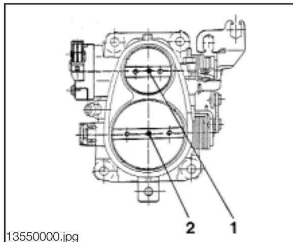
**Throttle Position Sensor:** A potentiometer is mounted on the throttle housing which provides the ECM with a voltage value (0-5v) that represents throttle angle position and rate of movement. The sensor receives its power supply from the ECM.
