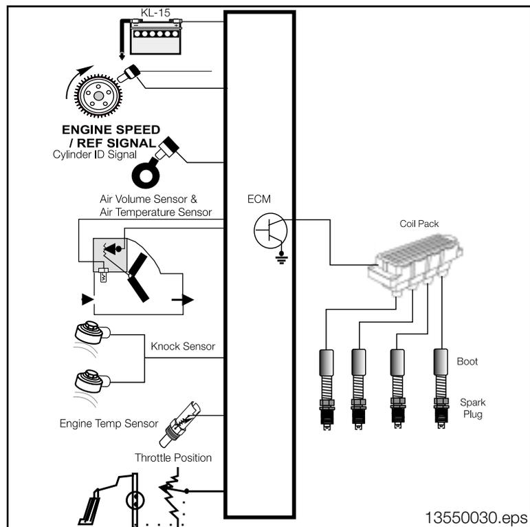
The timing will be advanced when the ECM observes low engine rpm and increasing throttle/air volume inputs (acceleration torque). As the throttle is opened, the ECM advances the timing based on engine acceleration and at what rate. The ECM will fully advance timing for the “full throttle” position indicating maximum acceleration (torque).
