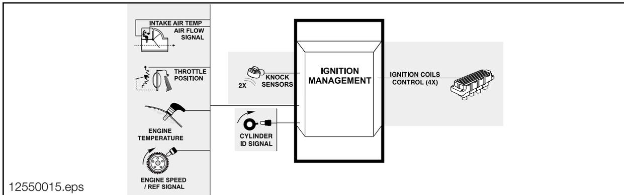
The ECM has a very “broad” range of ignition timing. This is possible by using a Direct Ignition System, or sometimes referred to as “Static Ignition System”. Reliability is also increased by having separate individual ignition circuits.
