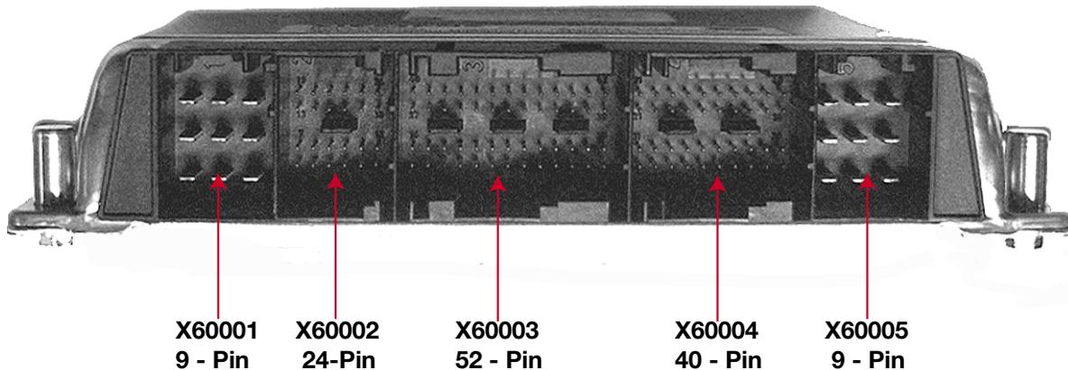
The 134 pin ECM is manufactured by Siemens to BMW specifications. The ECM is the SKE (standard shell construction) housing and uses 5 modular connectors. For testing, use the Universal Adapter Set (break-out box) Special Tool # 90 88 6 121 300.
