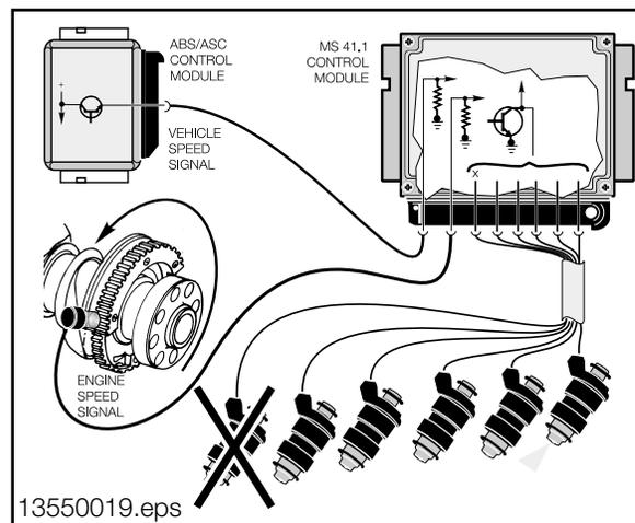
The ECM will also protect the Catalytic Converter by deactivating the injectors.
