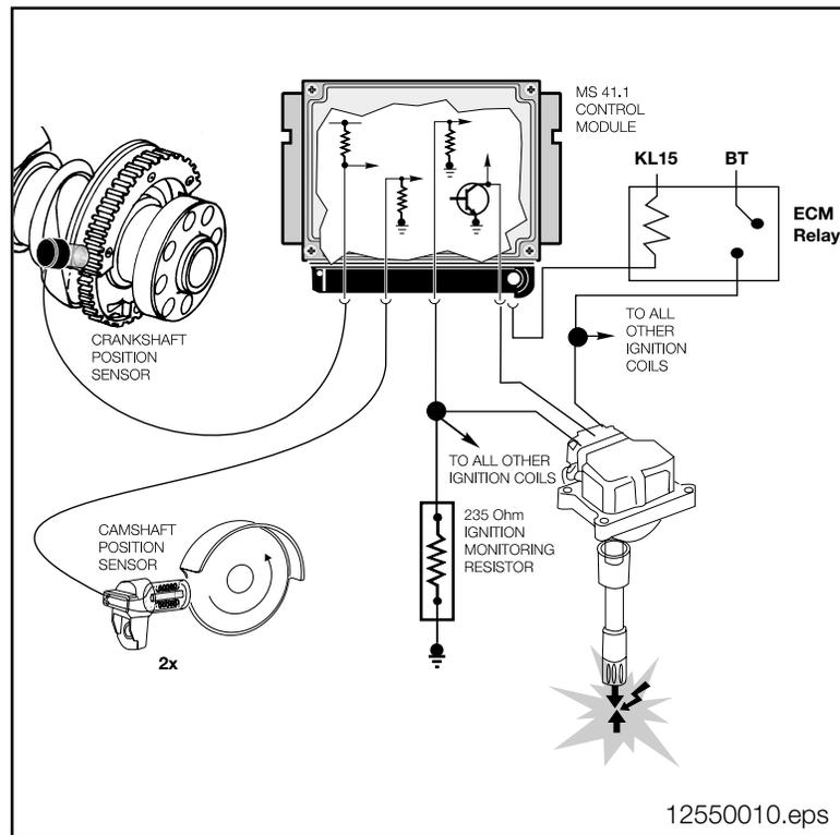
**Multiple Ignition Pulses** ensure good spark quality during engine start up. The ECM will activate the ignition coils 9 times (voltage dependent) per 720° of crankshaft revolution.
