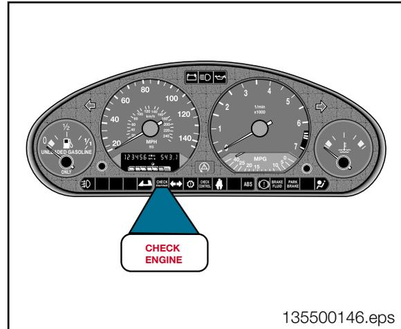
The ECM illuminates the “CHECK ENGINE” Light by activating a final stage transistor to supply a ground circuit (arrow). The light has voltage supplied whenever KL15 is switched “on”.
