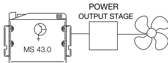
After the initial test has been performed, the fan is brought up to the specified operating speed. At 10% (sensing ratio) the fan runs at 1/3 speed. At a sensing ratio of between 90-95% the fan is running at maximum speed. Below 10% or above 95% the fan is stationary.
