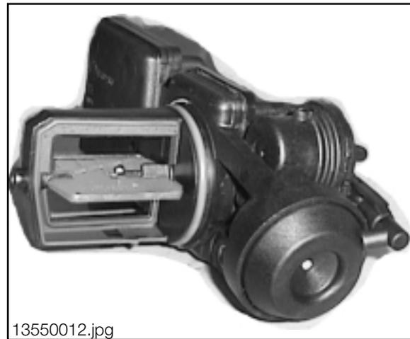
The ECM controls a solenoid valve for resonance flap activation. At speeds below 3750 RPM, the solenoid valve is energized and vacuum supplied from an accumulator closes the resonance flap. This channels the intake air through one resonance tube, but increases the intake velocity.
