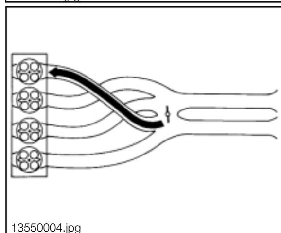
To accomplish this function, the M42 intake manifold incorporates a non-replaceable brass change over valve.
