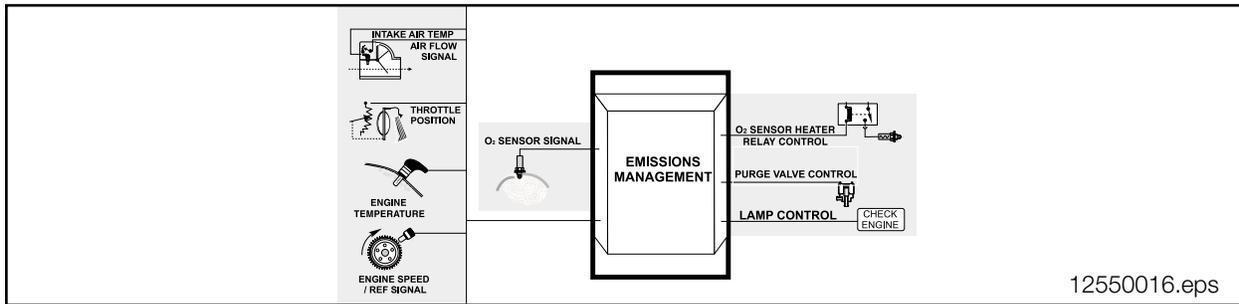
**Evaporative Emission Purging** is regulated by the ECM controlling the Evaporative Emission Valve. The Evaporative Emission Valve is a solenoid that regulates purge flow from the Active Carbon Cannister into the intake manifold. The ECM Relay provides operating voltage and the ECM controls the valve by regulating the ground circuit. The valve is powered closed and opened by an internal spring. The “purging” process takes place when:
