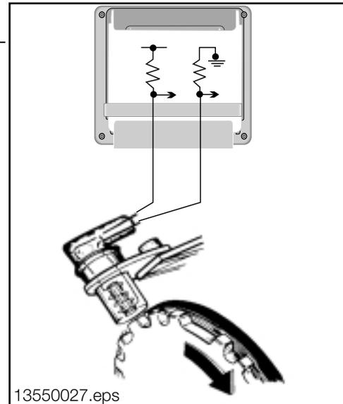
**Camshaft Position Sensor (Cylinder Identification):** The cylinder ID sensor (inductive pulse) input allows the ECM to determine camshaft position in relation to crankshaft position. It is used by the ECM to establish the “working cycle” of the engine for precise ignition timing. For details about the sensor, refer to the Fuel Management section.
