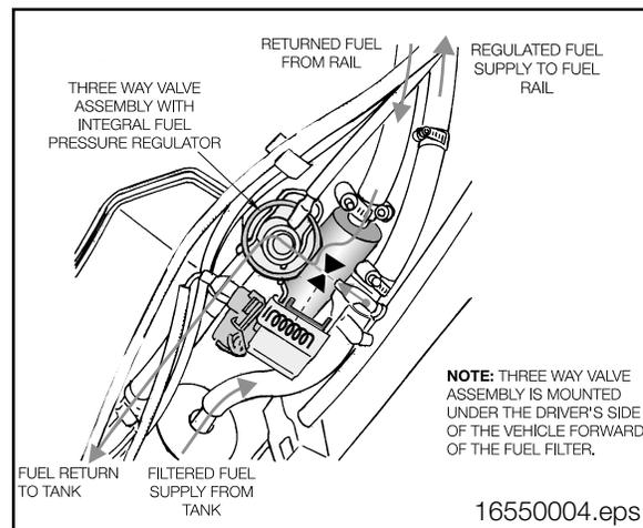
**MS42 Running Losses Fuel Supply:** The ECM controls the operation of the Running Losses Fuel Circuit by activating the by-pass solenoid. The solenoid is energized for 20 seconds on engine start up to supply full fuel volume to the fuel rail. After 20 seconds, the solenoid is deactivated and sprung closed (the by-pass is opened). This reduces the amount of fuel circulating through the fuel rail and diverts the excess to return through the fuel pressure regulator.
