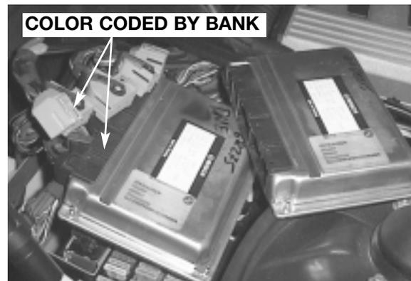
The correct Universal Adapter for the M5.2.1 application should be used (#90 88 6 121 300). This will ensure the pin connectors and the harness will not be damaged.
