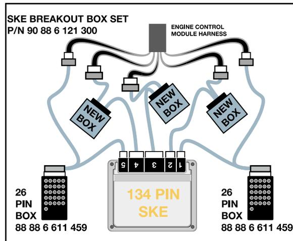
When installing the Universal Adapter to the ECM, make sure the ignition is switched off.
