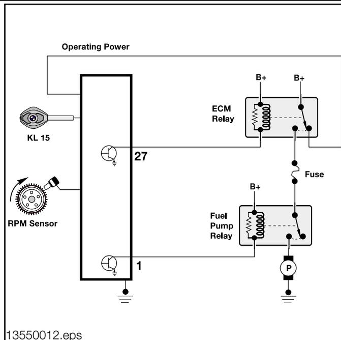
**The Fuel Injectors** will be opened by the ECM to inject pressurized fuel into the intake ports. The Fuel Injectors receive voltage from the Engine Control Module Relay. The ECM controls the opening by activating the ground circuit for the Solenoid Windings. The ECM will vary the duration (in milli-seconds) of “opening” time to regulate the air/fuel ratio.
