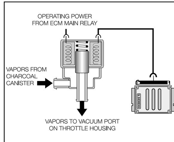
The Evaporative Emission Valve is opened in stages to moderate the purging.
