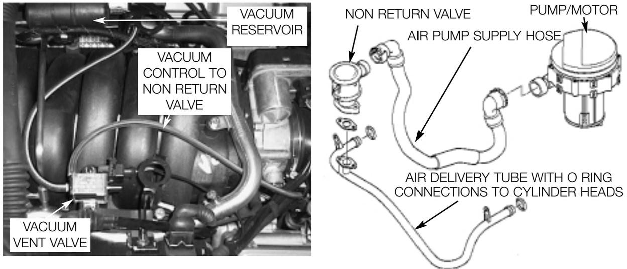
The ME7.2 control unit controls the vacuum vent valve and the secondary air injection pump relay separately but simultaneously.
