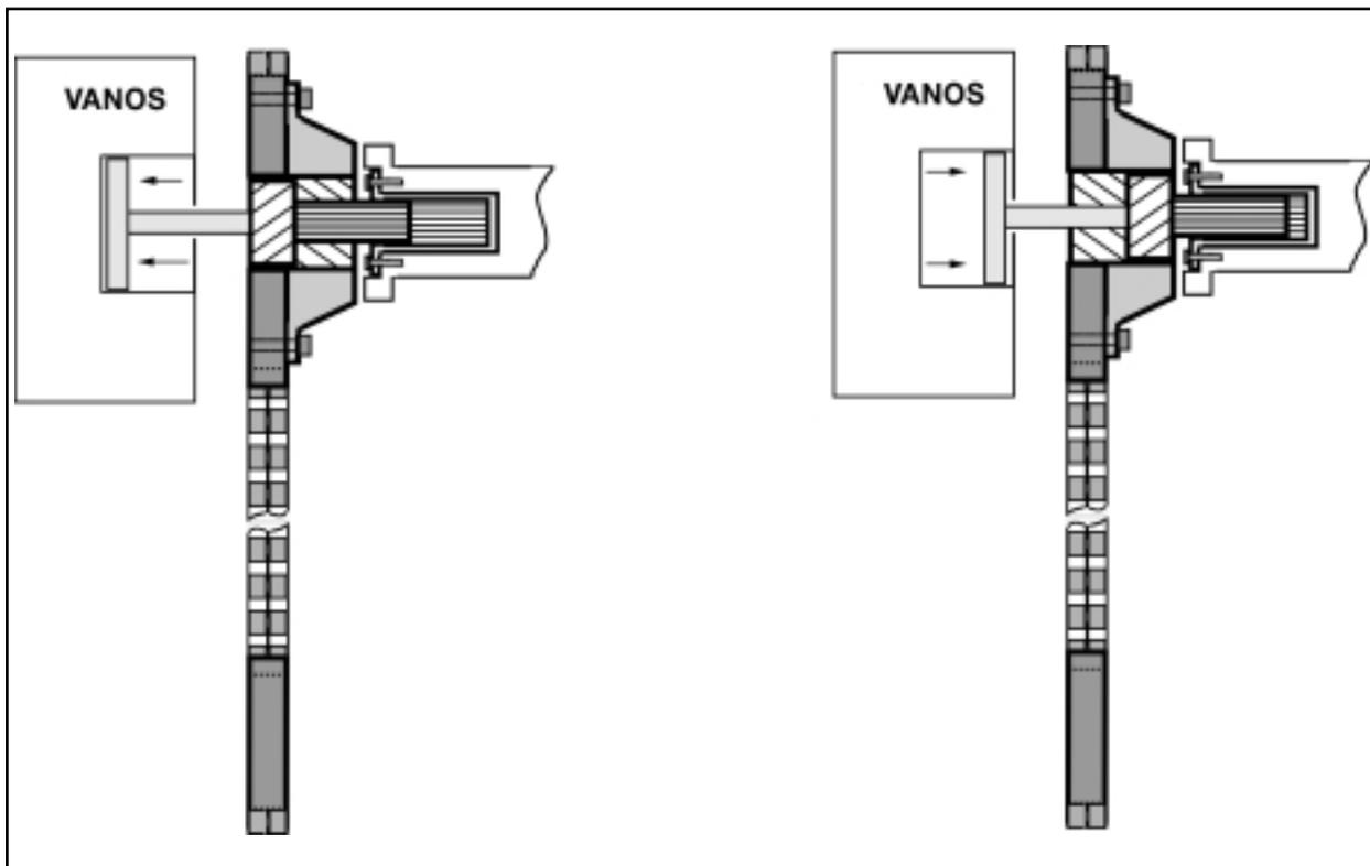
The operation of the VANOS solenoid is monitored in accordance with the OBD II requirements for emission control. The ECM monitors the final stage output control and the signal from the Camshaft Position Sensors for VANOS operation.
