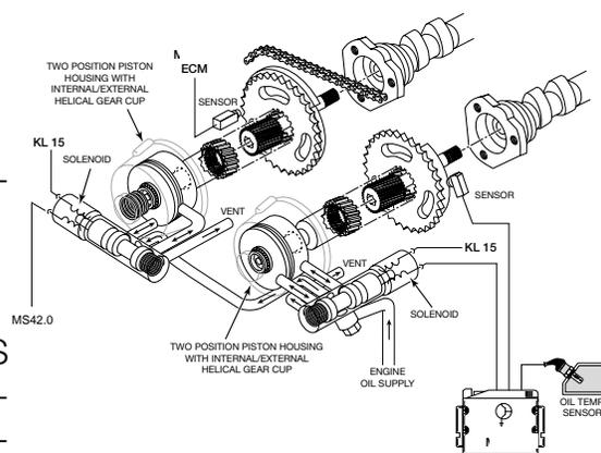
The exhaust cam sensor is used for VANOS position control of the exhaust cam. If these sensors fail there are no substitute values, the system will operate in the failsafe mode with no VANOS adjustment. The engine will still operate, but torque reduction will be noticeable.
