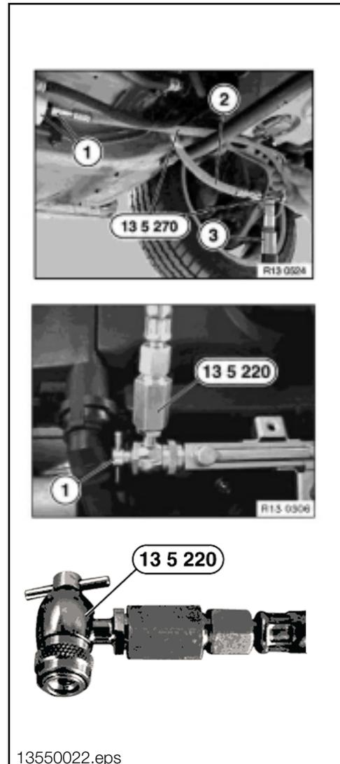
Later production fuel rails are equipped with a threaded adapter fitting (1).
