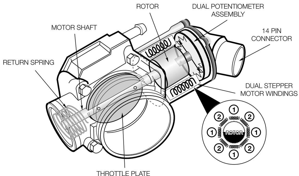
The dual feedback potentiometers signal the movement and position of the throttle plate to each processor. The two potentiometers have separate power and ground circuits to ensure the reliability of their operation.
