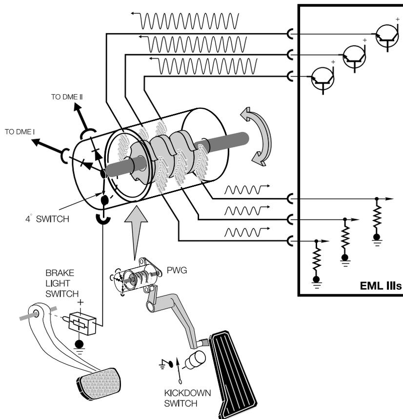
The amplitude is decreased as the pedal is pressed down.
