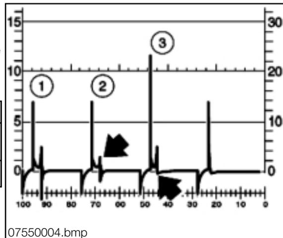
No Sparking Voltage Line (Single Cylinder Displayed)
