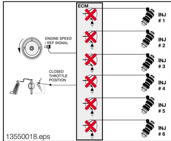
When the engine rpm approaches idle speed, the injection ms value is increased (cut-in) to prevent the engine from stalling. The cut-in rpm is dependent upon the engine temperature and the rate of deceleration. This function can be observed as displayed on the Fuel Economy (MPG) gauge.
