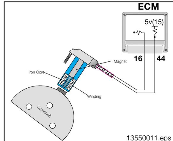
If the ECM detects a fault with the Cylinder ID Sensor, the “CHECK ENGINE” Light will be illuminated and the system will still operate based on the Crankshaft Position/RPM Sensor. Upon a restart, a slight change in driveability could occur because the ECM will activate Parallel Fuel Injection, all of the injectors will be activated at the same time.
