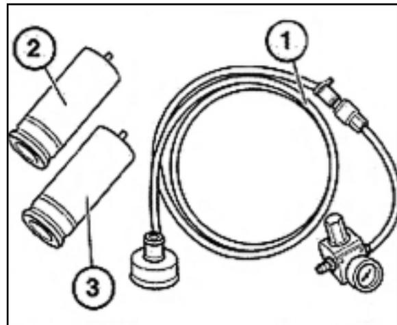
This Special Tool Set #90 88 6 161 160 will also be required to “cap off” the air filter and Evaporative Emission Valve hose when performing the Leakage Diagnosis Test.
