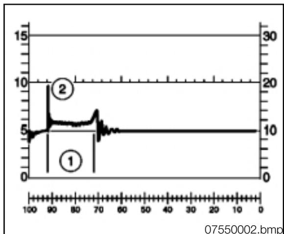
Evaluation of Ignition Voltage Peaks at Idle Speed (Multiple Cylinders Displayed).
