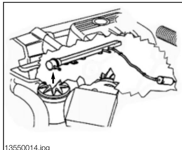
**Bosch Fuel Injectors:** The Fuel Injectors are electronically controlled solenoid valves that provide precise metered and atomized fuel into the engine intake ports. The Fuel Injector Valve consists of:
