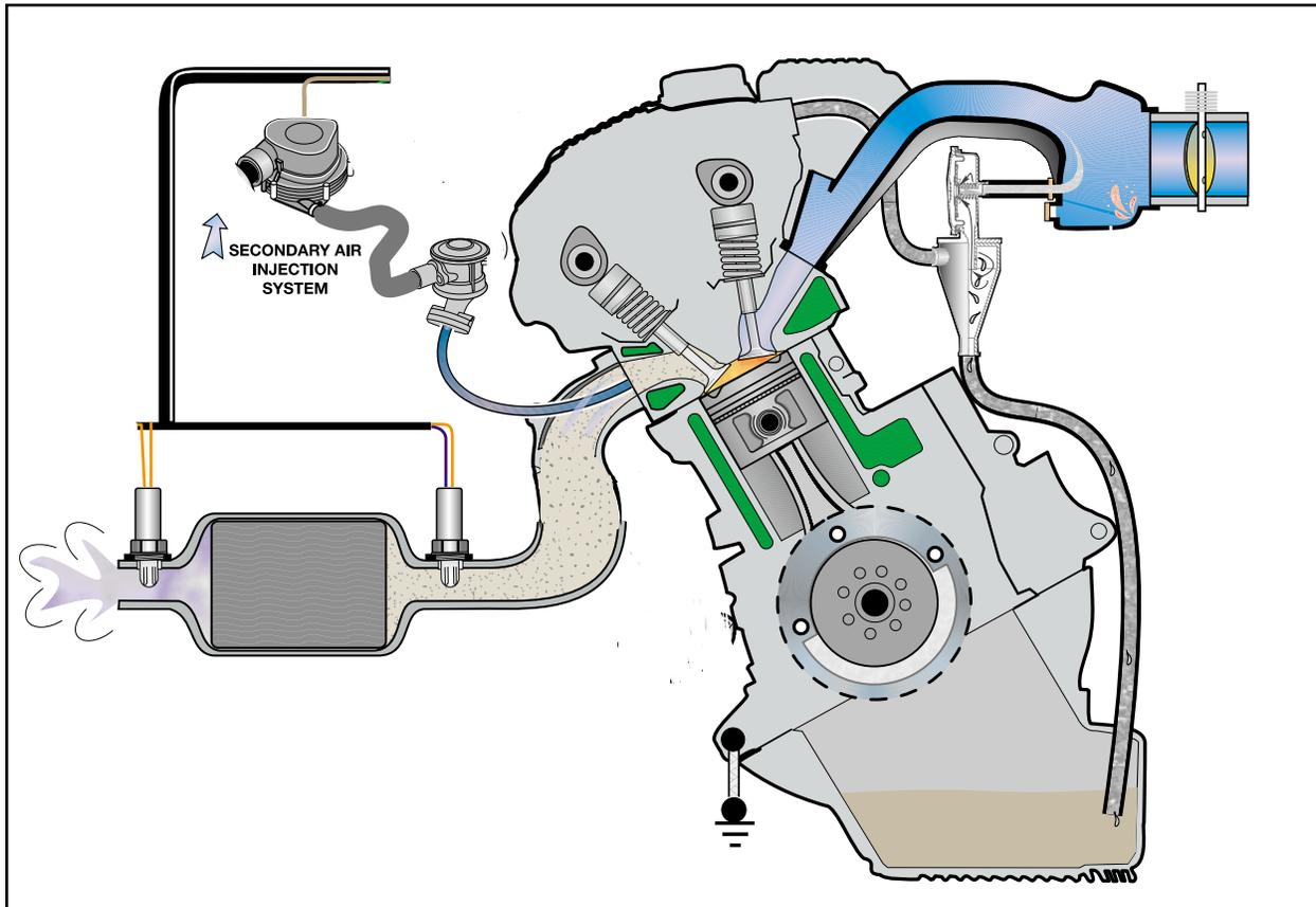
**Exhaust Emissions:** The combustion process of a gasoline powered engine produces Carbon Monoxide (CO), Hydrocarbons (HC) and Oxides of Nitrogen (NO<sub>x</sub>).
