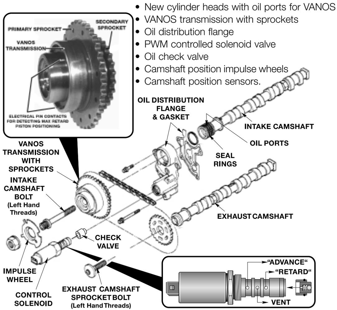
**VANOS CONTROL SOLENOID & CHECK VALVE:** The VANOS solenoid is a two wire, pulse width modulated, oil flow control valve. The valve has four ports;
