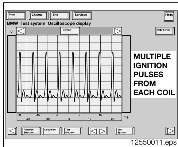
The multiple pulsing switches to single pulse when:
