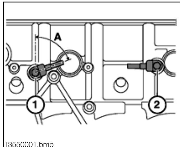
**Crankshaft Position/RPM Sensor:** This sensor provides the crankshaft position and engine speed (RPM) signal to the ECM for ignition activation and correct timing. For details about the sensor, refer to the Fuel Management section.
