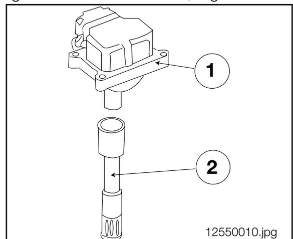
**Spark Plugs:** The spark plugs introduce the ignition energy into the combustion chamber. The high voltage “arcs” across the air gap in the spark plug from the positive electrode to the negative electrode. This creates a spark which ignites the combustible air/fuel mixture.
