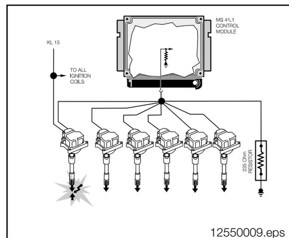
If there is a fault in the secondary ignition, testing should include:
