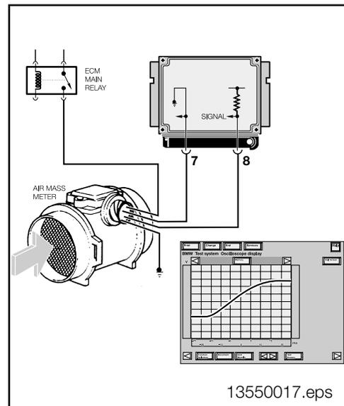
**NOTE:** The Siemens 2 Type B designation simply indicates that the sensor is smaller in design. The mass air meter has different diameters based on engine application. The HFM is non-adjustable.
