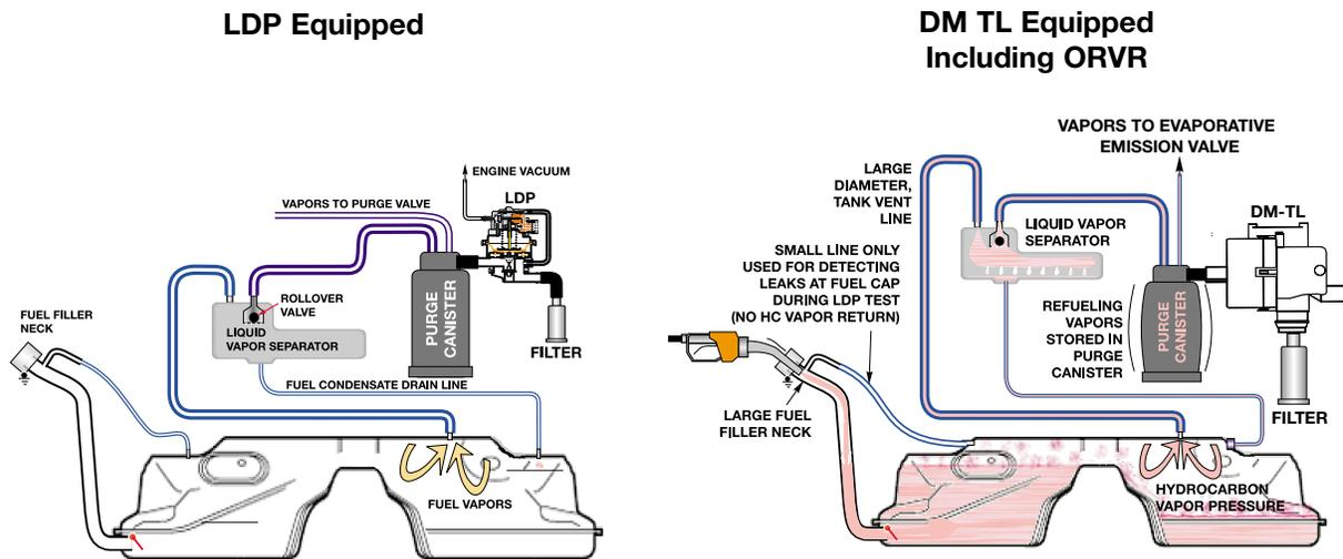
**Evaporative Emissions:** The control of the evaporative fuel vapors (Hydrocarbons) from the fuel tank is important for the overall reduction in vehicle emissions. The evaporative system has been combined with the ventilation of the fuel tank, which allows the tank to breath (equalization). The overall operation provides:
