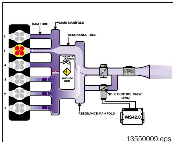
The resonance “wave”, along with the intake velocity, enhances cylinder filling.
