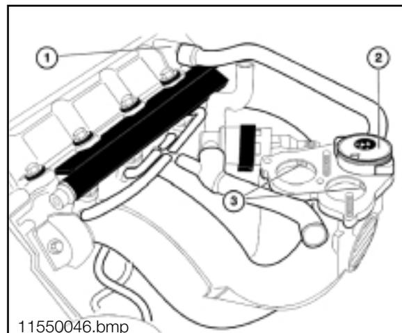
At idle when the intake manifold vacuum is high, the vacuum decrease the valve opening and only allows a small amount of crankcase vapors to be drawn into the intake manifold.
