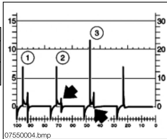
No Sparking Voltage Line (Single Cylinder Displayed)
