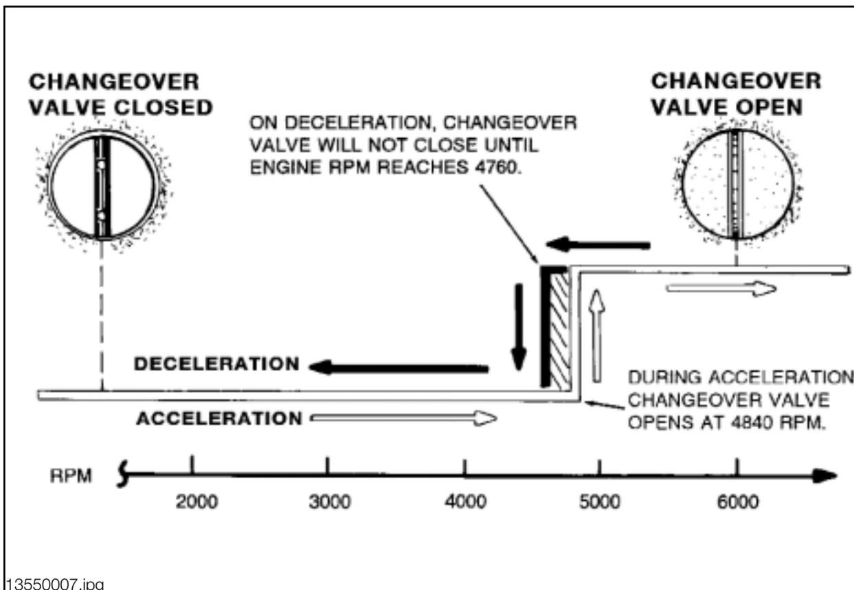
If there is a defect in this system, the Changeover Valve will be opened to ensure intake air availability for maximum power (short pipe affect). The Vacuum Motor and valve shaft are both spring loaded to open the Changeover Valve if vacuum is not applied.
