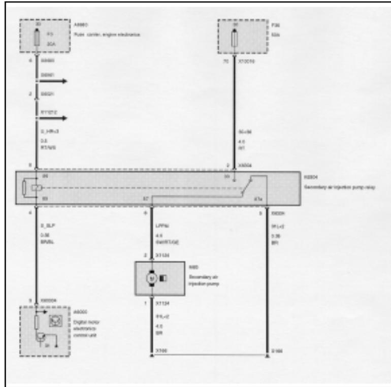
**Secondary Air Injection Monitoring** is performed by the ECM via the use of the pre-catalyst oxygen sensors. Once the air pump is active and is air injected into the exhaust system the oxygen sensor signals will indicate a lean condition (up to 16 seconds).
