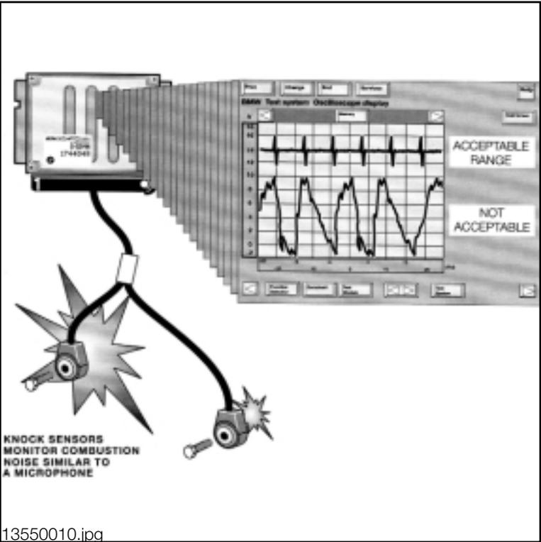
If a fault is detected with the Knock Sensor(s) or circuits, the ECM deactivates Knock Control. The “CHECK ENGINE” Light will be illuminated, the ignition timing will be set to a conservative basic setting (to reduce the risk of detonation) and a fault will be stored.
