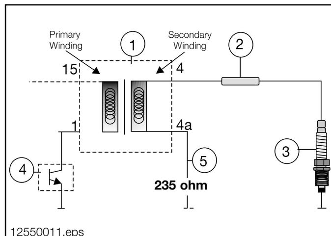
The Coil Assembly contains two copper windings insulated from each other. One winding is the primary winding, formed by a few turns of thick wire. The secondary winding is formed by a great many turns of thin wire.
