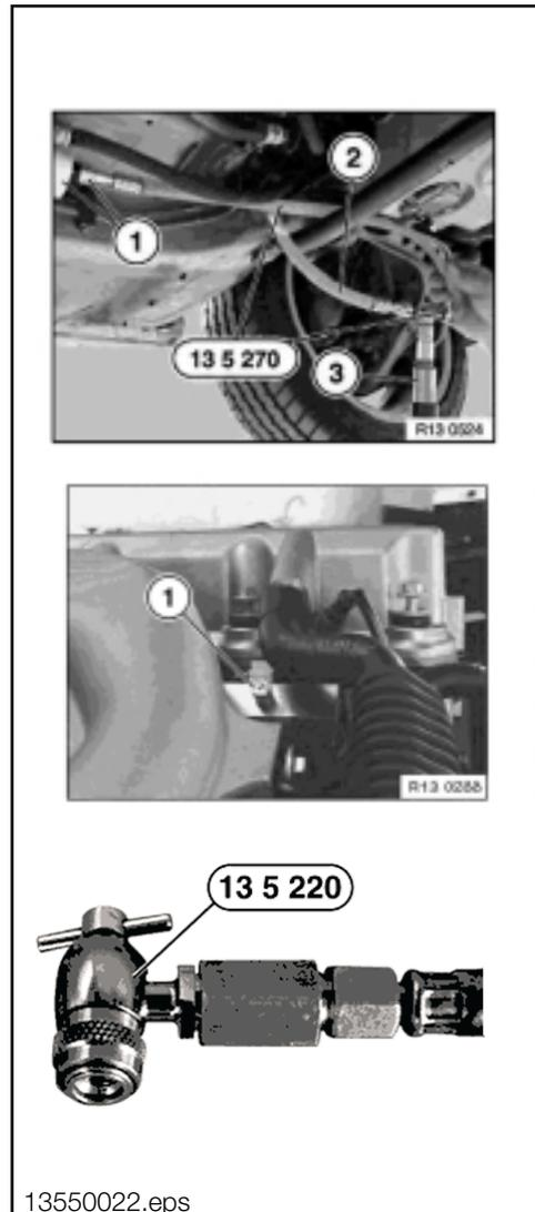
When testing the fuel injectors for leakage, use Special Tool #88 88 5 000 362. Leak testing the fuel injectors is one of the diagnostic steps listed in "Long Cranking Times" S.I. #13 08 90 (3096). This tool pressurizes the injectors with air and the injector tips are submerged in water. If air bubbles are present, this indicates the leaking injector(s).
