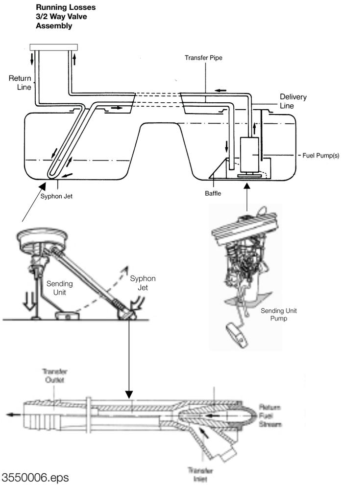
**Fuel Pump:** The electric fuel pump supplies constant fuel volume to the injection system. This system uses a single submersible (in the fuel tank) pump. The inlet is protected by a mesh screen.
