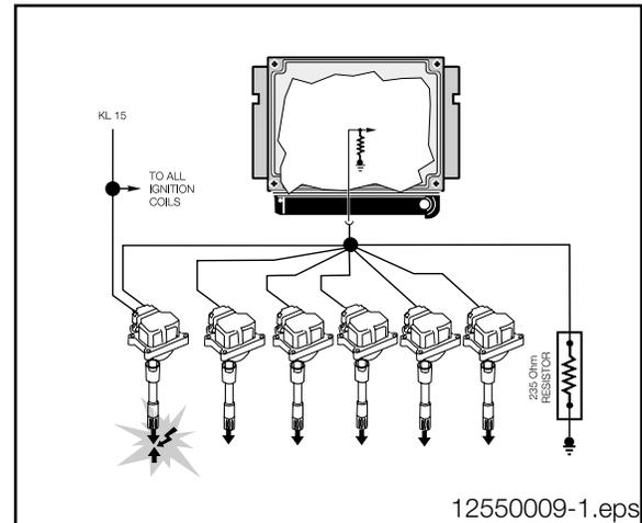
As the secondary magnetic field collapses, a voltage spike is induced in the windings. The ECM monitors the voltage drop across the resistor as an indication of coil firing. After the ECM activates the primary ignition, this feedback signal (**Terminal 4a Signal**) is confirmation that secondary ignition took place. The ECM measures the duration of time it takes the voltage drop for each ignition coil to dissipate below two volts. The time scale constantly changes based on engine rpm.
