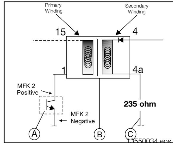
ECM Final Stage transistor activation. This test function is found under the Oscilloscope Preset list - "Ignition Signal Primary" (normal Terminal 1 Signal shown on the right).
