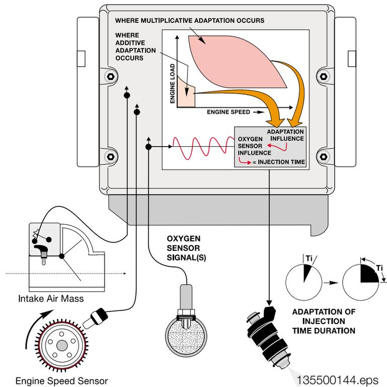
**Adaptation Values** are stored by the ECM in order to maintain an "ideal" air/fuel ratio. The ECM is capable of adapting to various environmental conditions encountered while the vehicle is in operation (changes in altitude, humidity, ambient temperature, fuel quality, etc.).
