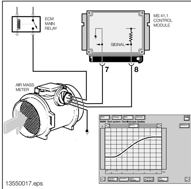
**NOTE:** Visually inspect the sensor for damaged, missing or blocked screens. The screens affect air flow calibration. Also inspect the sealing rings where the sensor inserts in the air filter housing and intake boot. Ensure the pin connections are tight.
