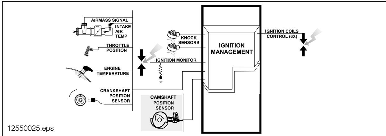
**Ignition Coils:** The high voltage supply required to ignite the mixture in the combustion chambers is determined by the stored energy in the ignition coils. The stored energy contributes to the ignition duration, ignition current and rate of high voltage increase. The Coil circuit including primary and secondary components consists of:
