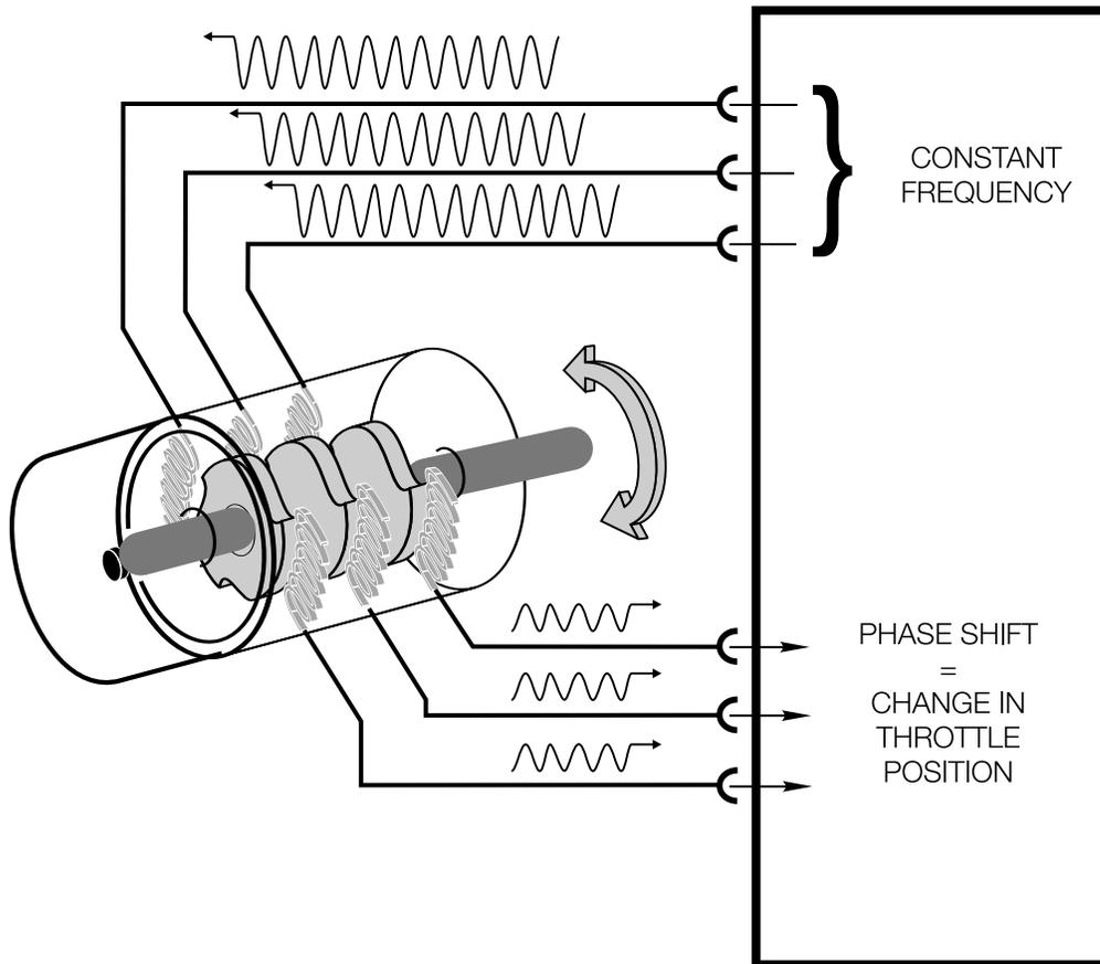
The changing amplitude value is a measure of accelerator pedal movement. The EML control module is programmed to recognize pedal movement from 0° (idle) to 99° (WOT) based on the changing voltage signal.
