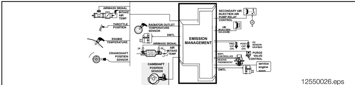
**The MS42 Evaporative Leakage Detection** uses a Leak Diagnosis Pump (LDP) to pressurize the fuel tank and the evaporative emission system (approx. 25mb.). The LDP equipped system is capable of detecting a leak as small as 0.5 mm. The LDP is replaceable as a complete component. The vacuum supply line (required for pump operation) is in the wiring harness from the engine compartment to the rear of the vehicle.
