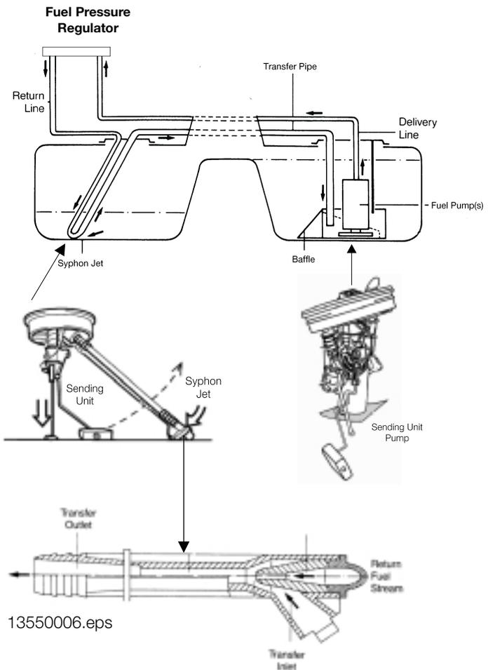
**Fuel Pump:** The electric fuel pump supplies constant fuel volume to the injection system. This system uses a single submersible (in the fuel tank) pump. The inlet is protected by a mesh screen.
