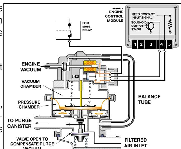
During every engine cold start the LDP solenoid is energized by the ECM. Engine manifold vacuum enters the upper chamber of the LDP to lift up the spring loaded diaphragm.
