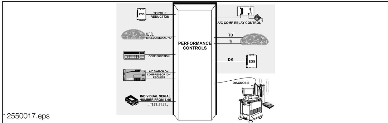
**Engine Speed Signal (TD):** is produced by the ECM as an output function. The TD signal is a processed square wave signal that indicates engine rpm. The signal is made available to other control modules including the Instrument Cluster, EWS and the 20 pin Diagnostic Socket.
