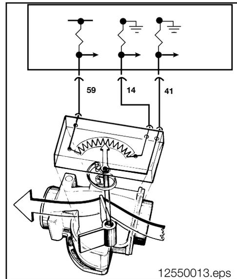
**NOTE:** The Air Flow Volume Sensor is non-adjustable.
