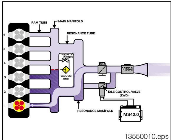
As the intake air is flowing into cylinder #1, the intake valves will close.
