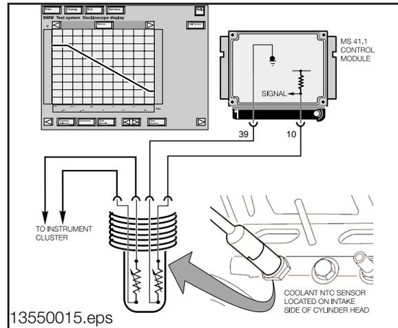
If the Coolant Temperature Sensor input is faulty, a fault code will be set the ECM will assume a substitute value (80° C) to maintain engine operation.
