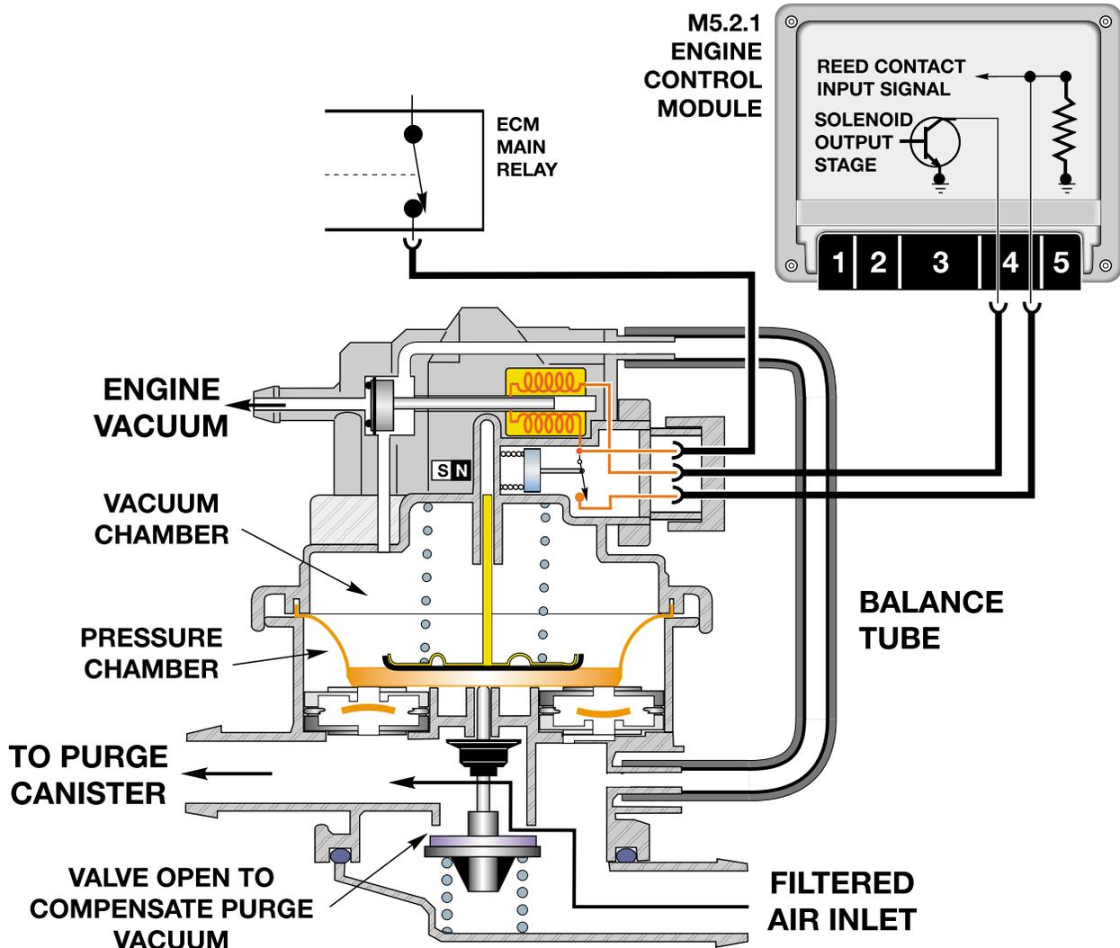
A fault code can be recorded by each ECM indicating an evaporative system leak. Upon test completion, the ECM releases the ground path to the LDP and the internal spring pushes the diaphragm for the “full down stroke”.
