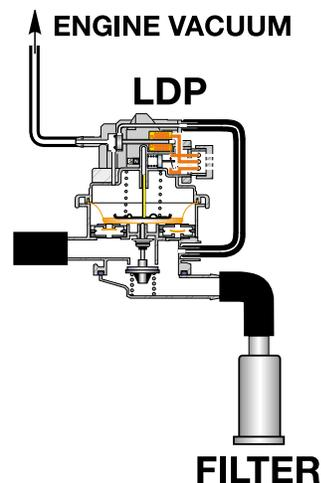
The ECM monitors the length of time it takes for the reed switch to open, which is opposed by pressure under the diaphragm in the lower chamber. If this component/circuits are defective, a fault code will be set and the "Malfunction Indicator Light" will illuminate when the OBD II criteria is achieved.
