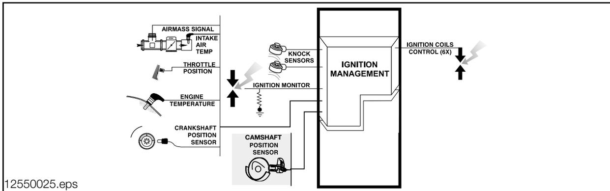
The ECM has a very “broad” range of ignition timing. This is possible by using a Direct Ignition System, or sometimes referred to as “Static Ignition System” (RZV). Reliability is also increased by having separate individual ignition circuits.
