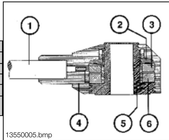
A piezo-ceramic ring is clamped between a seismic mass and the sensor body. When the seismic mass senses vibration (flexing), it exerts a force on the piezo-ceramic element. Opposed electrical charges build up on the upper and lower ceramic surfaces which generates a voltage signal. The acoustic vibrations are converted into electrical signals. These low voltage signals are transmitted to the ECM for processing.
