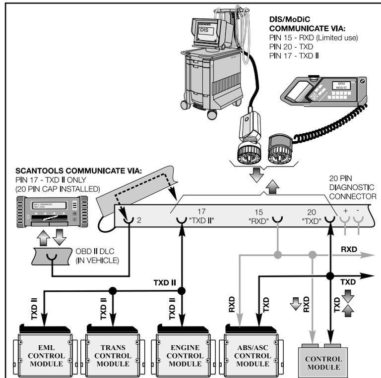
The DLC Connector bridging cap is marked **"OBD II"** and is found:
