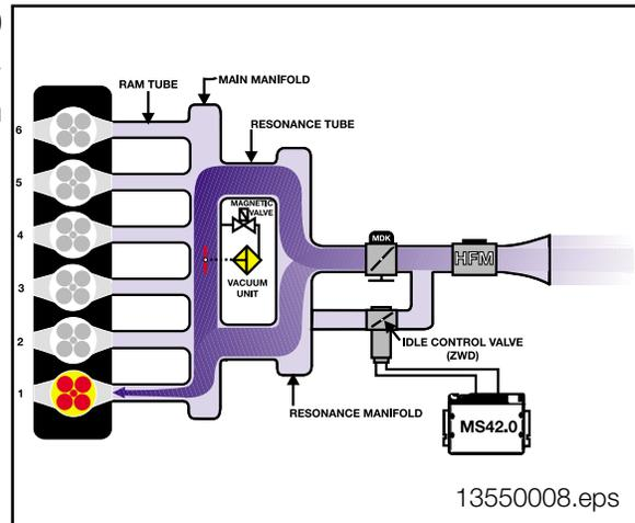
• #5 Cylinder Intake Valve Open - Intake air drawn from both resonance tubes. Mid to High Range RPM (>3750 RPM).
