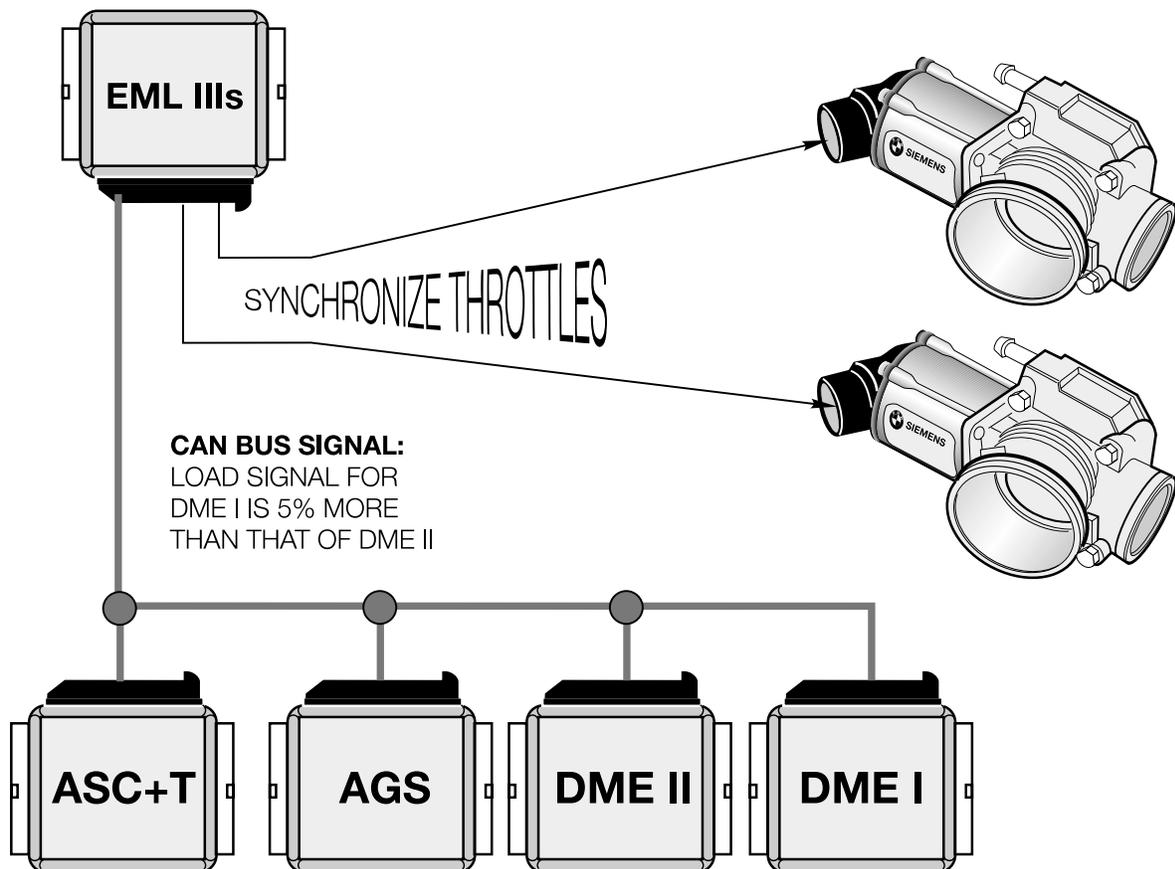
The EML control module processes the load signals from the two DME control modules. If a difference exists, the EML will adjust the DK motors to achieve equal air throughput on both banks. If the load difference is greater than 10%, the synchronization will not take place and a fault is stored in the memory.
