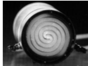
The heating coils are provided operating current from an E-CAT control module located under the passenger seat. The coils are connected to the E-Cat control module by high amperage cables. The cables pass through a rubber grommet on the passenger side floor to the E-CAT module location.
