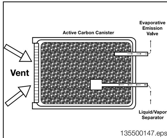
**Evaporative Emission Valve:** This ECM controlled solenoid valve regulates the purge flow from the Active Carbon Canister into the intake manifold (located next to the Air Volume Mass Meter).
