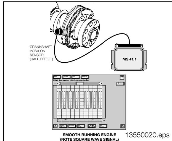
The crankshaft position sensor is monitored as part of OBD II requirements for Misfire Detection. If this input is faulty, the ECM will operate the engine (limited driveability) from the Camshaft Sensor input. A fault with this input will produce the following complaints:
