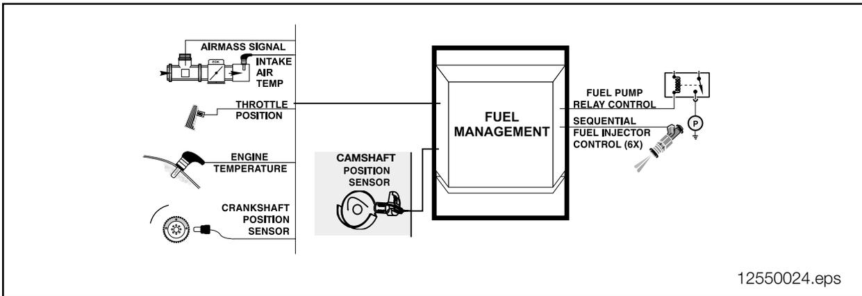
**The Fuel Pump** will be activated when the ignition (KL15) is switched “on” and the ECM supplies a ground circuit to activate the Fuel Pump Relay. The Fuel Pump Relay supplies operating power to the in-tank mounted fuel pump. This is a momentary activation to “pressurize” (prime) the fuel system.
