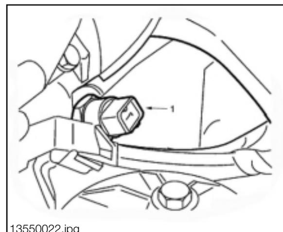
If the Coolant Temperature Sensor input is faulty, the “CHECK ENGINE” Light will be illuminated and the ECM will assume a substitute value (80° C) to maintain engine operation.
