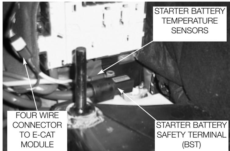
Once the E-CATs are activated, the control module simultaneously provides the output control signal to the dual battery isolation switch (signal KATON) requesting the switch which opens the circuit between the starter battery and vehicle circuit battery. This ensures the E-Cat's operating power is supplied only from the starter battery (detailed description of two battery system further on).
