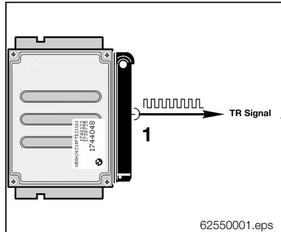
**Throttle Position (DKV) for EGS:** is the output signal to the EGS Control Module (if equipped). The DKV signal is a pulse width modulated signal directly proportional to the linear throttle position sensor input signal.
