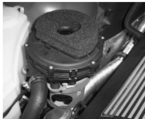
The Air Injection Inlet Valve mounts directly to the cylinder head, with a passageway machined through the head. This eliminates the external Air Injection manifold distribution pipes to the exhaust manifolds.
