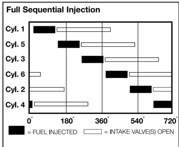
**The Injector “open” Time** to maintain engine operation after it has been started is determined by the ECM (programming). The ECM will calculate the injection “timing” based on a combination of the following inputs:
