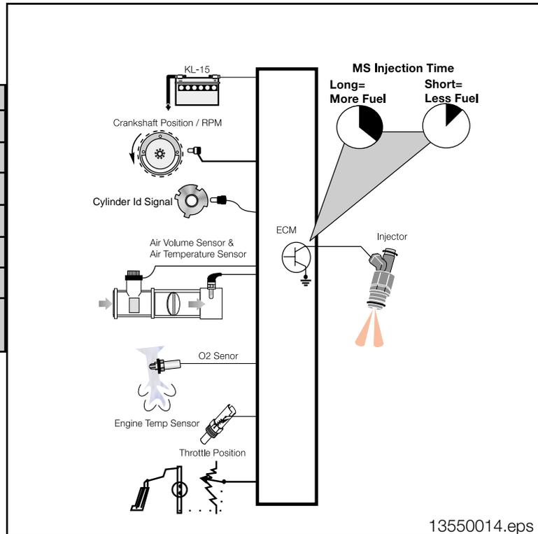
The injection ms value will be regulated based on battery voltage. When cranking, the voltage is low and the ECM will increase the ms value to compensate for injector “lag time”. When the engine is running and the battery voltage is higher, the ECM will decrease the injection ms value due to faster injector reaction time.
