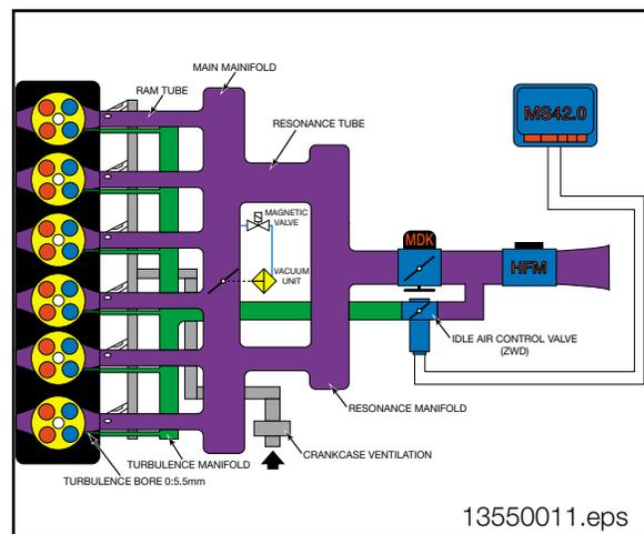
Under certain engine operating parameters, the MDK/EDK throttle control and the Idle Air Actuator are operated simultaneously. This includes all idling conditions and the transition from off idle. As the request for load increases, the idle valve will remain open and the MDK/EDK will supply any additional air volume required to meet the demand.
