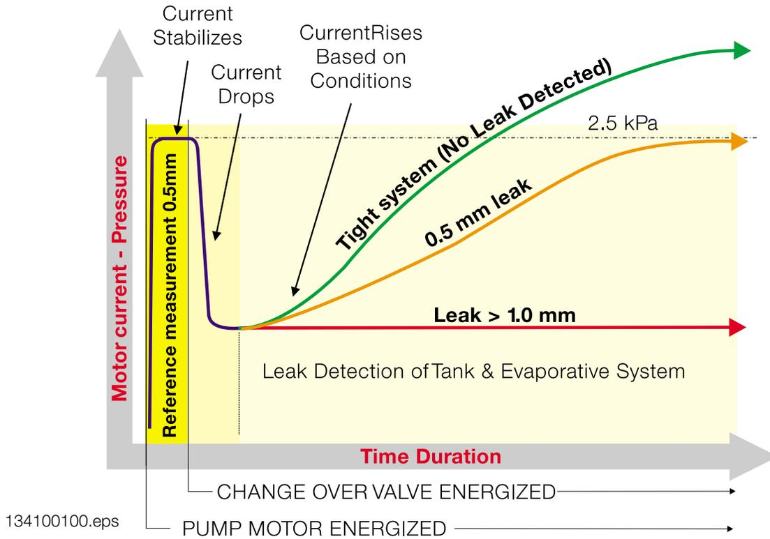
If the ECM detects a leak, a fault will be stored and the “Malfunction Indicator Light” will be illuminated. Depending on the amperage measurement detected by the ECM, the fault code displayed will be “small leak” or “large leak”.
