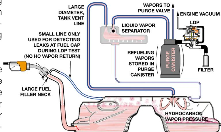
The HC is stored in the charcoal canister, and the system can then “breathe” through the LDP and the air filter.
