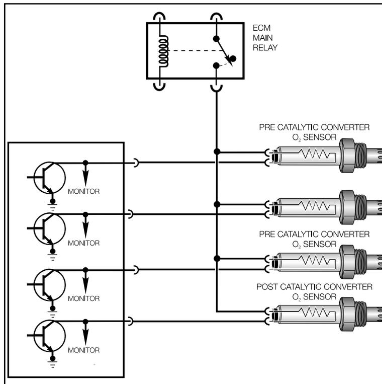
**Catalytic Converter Monitoring:** The efficiency of catalyst operation is determined by evaluating the oxygen consumption of the catalytic converters using the pre and post oxygen sensor signals. A properly operating catalyst consumes most of the O<sub>2</sub> (oxygen) that is present in the exhaust gas (input to catalyst). The gases that flow into the catalyst are converted from CO, HC and NO<sub>x</sub> to CO<sub>2</sub>, H<sub>2</sub>O and N<sub>2</sub> respectively.
