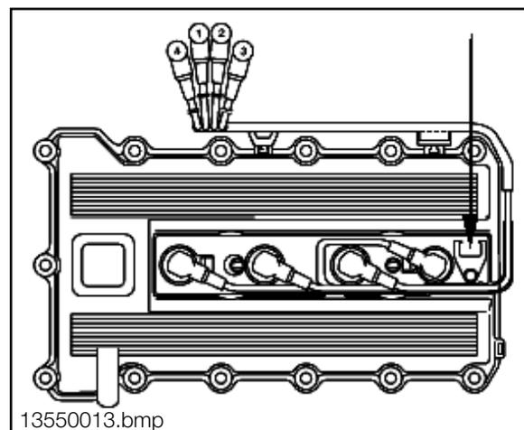
**Spark Plugs:** The spark plugs introduce the ignition energy into the combustion chamber. The high voltage “arcs” across the air gap in the spark plug from the positive electrode to the negative electrode. This creates a spark which ignites the combustable air/fuel mixture.
