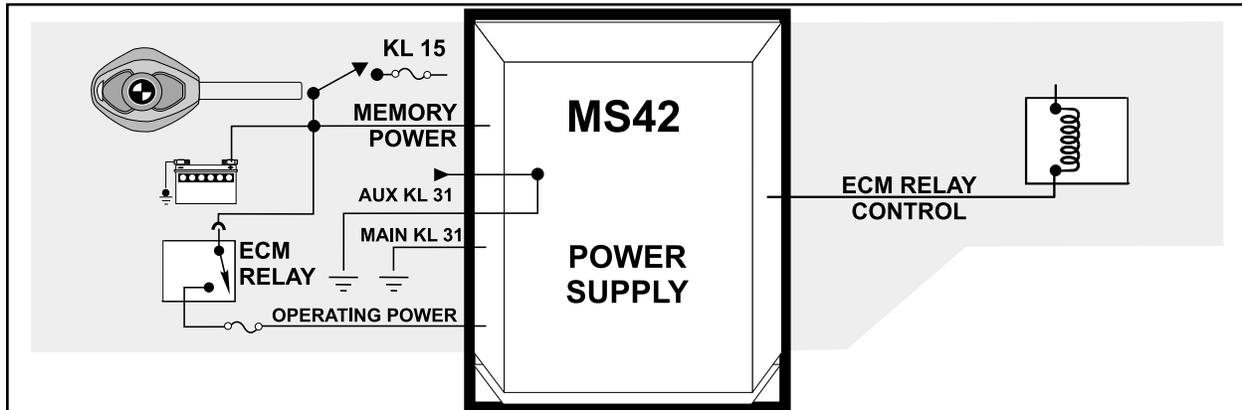
**KL30 - Battery Voltage:** B+ is the main supply of operating voltage to the ECM.
