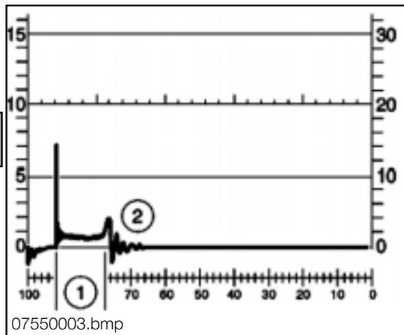
Evaluation of Ignition Voltage Peaks at Idle Speed (All Cylinders Displayed).
