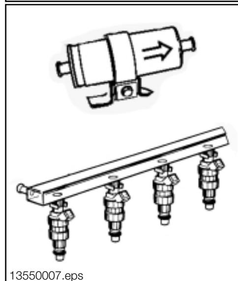
**Fuel Pressure Regulator:** The Fuel Pressure Regulator maintains a constant “pressure differential” for the fuel injectors.
