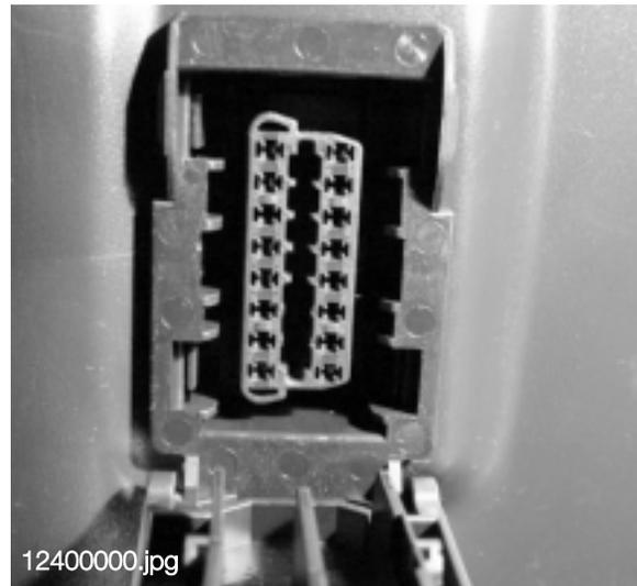
The cap to the OBD II connector contains a bridge that links KL 30 to TXD and TXD II. This is to protect the diagnostic circuit integrity and prevent erroneous faults from being logged.
