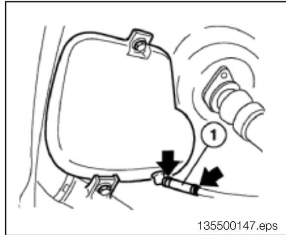
**Active Carbon Cannister:** As the hydrocarbon vapors enter the canister, they will be absorbed by the active carbon. The remaining air will be vented to the atmosphere through the end of the canister allowing the fuel tank to “breathe”.
