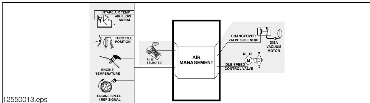
**Throttle Valve:** The mechanical throttle valve regulates the intake air flow and it is linked by a cable to the accelerator pedal.
