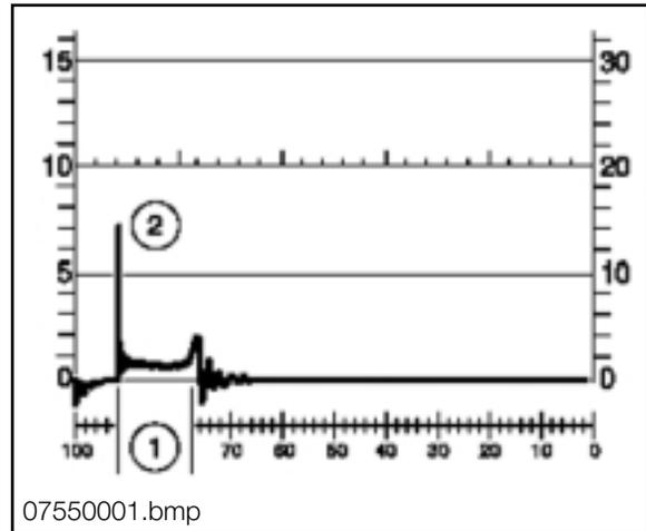
**Multiple Ignition Pulses** ensure good spark quality during engine start up. The ECM will activate the ignition coils 9 times per 720° of crankshaft revolution.
