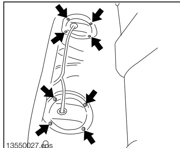
The passenger side allows access to the fuel pump/sending unit.
