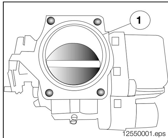
The throttle assembly for the **MS43** system is referred to as the **EDK**. The EDK is distinguished by:
