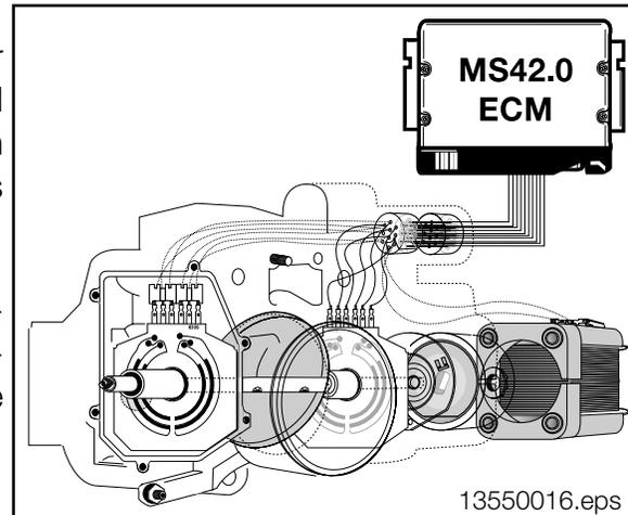
**EDK:** The MS43 ECM powers the EDK motor using pulse width modulation for opening and closing the throttle plate. The throttle plate is also closed by an integrated return spring.
