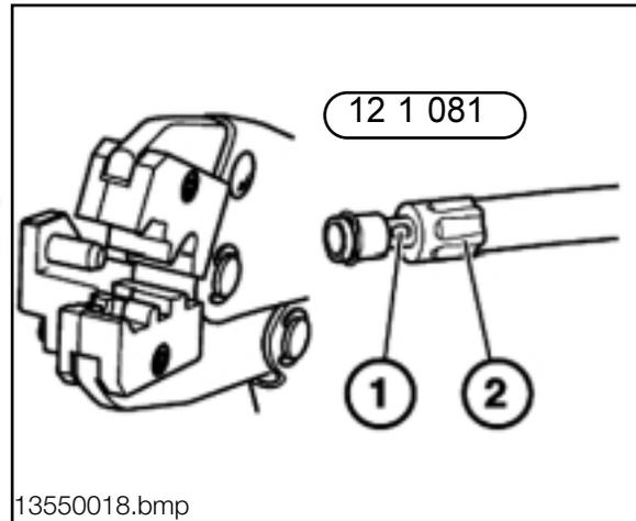
The connector with ignition cable should be installed into the Resistive Adapter Boot with Special Tools #12 1 087 and #12 1 086 to ensure the connector properly “seats”.
