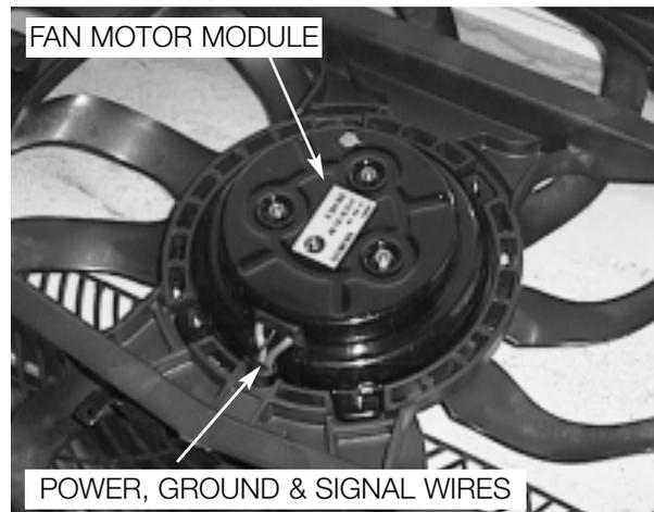
When the over temperature light in the instrument cluster is on (120°C) the fan is run in the overrun function. This signal is provided to the DME via the CAN bus. When this occurs the fan is run at a frequency of 10 Hz.
