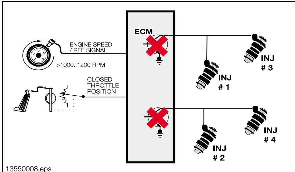
As the throttle is closed during deceleration, the ECM decreases the injection ms value (fuel shut off) if the rpm is above idle speed (coasting). This feature decreases fuel consumption and lowers emissions.
