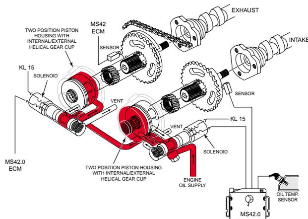
The dual VANOS in conjunction with the variable intake manifold provides an additional emission control feature.
