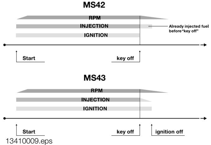
When **KL15** is switched “off” the ECM operating voltage is removed.
