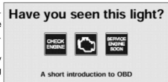
This light informs the driver of the need for service, NOT of the need to stop the vehicle. A blinking or flashing dashboard light indicates a rather severe level of engine misfire.
