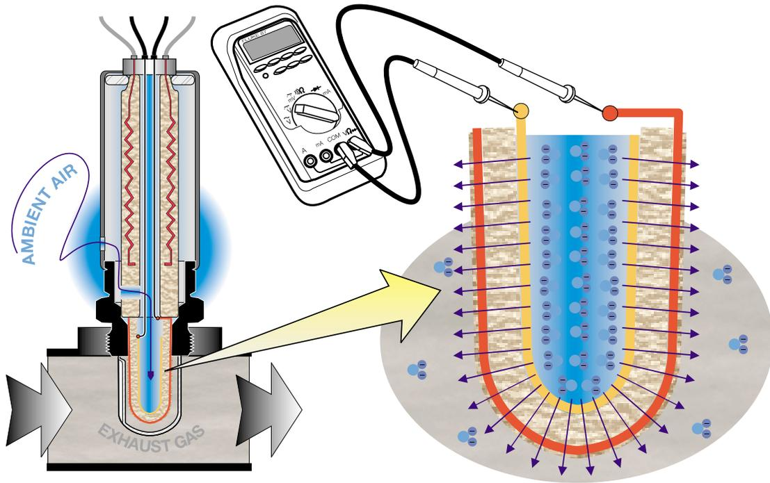
If the exhaust has a lower oxygen content (rich mixture), there will be a large ion “migration” through the sensor generating a higher voltage (950 mV).
