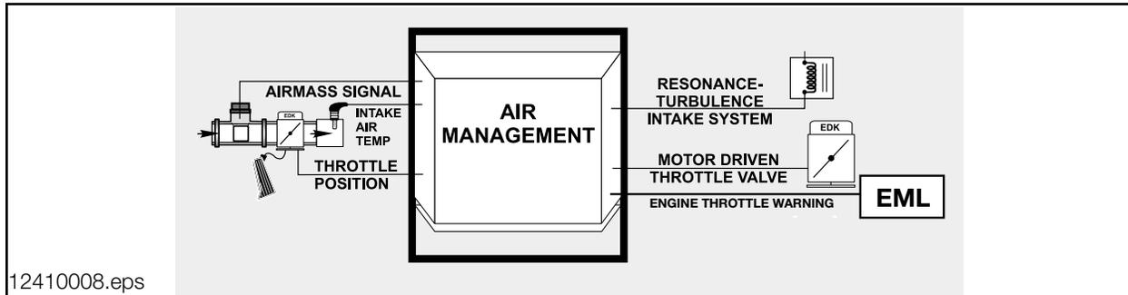
**The Accelerator Pedal Position (PWG)** is monitored by the ECM for pedal angle position and rate of movement. As the accelerator is moved, a rising voltage signal from the potentiometers/Hall sensors requests acceleration and at what rate. The ECM will increase the volume of fuel injected into the engine, advance the ignition timing and open the Throttle Valve and/or Idle Air Actuator.
