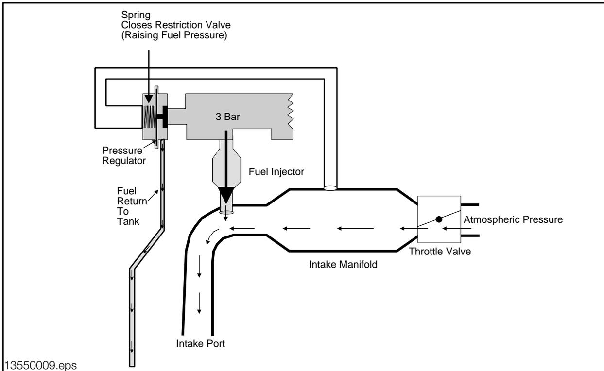
By maintaining constant Fuel Pressure Differential through vacuum sensing (engine load), the ECM can then regulate volume and mixture by the length of time the injectors are open (duration).
