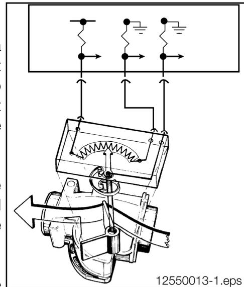
**Air Temperature:** This signal allows the ECM to make a calculation of air density. The sensor is located in front of the measuring flap. For details about the sensor, refer to the Air Management section.
