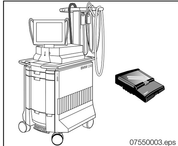
The correct Universal Adapter for the MS42/MS43 application should be used (#90 88 6 121 300). This will ensure the pin connectors and the harness will not be damaged.
