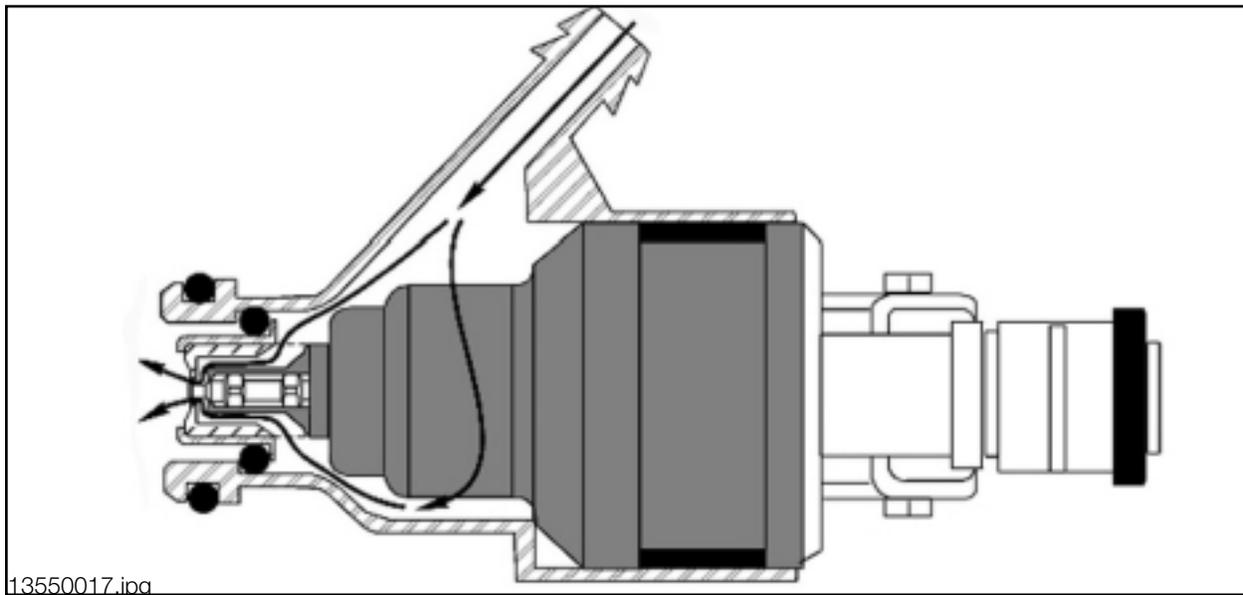
The Air Shrouded Injectors incorporate a hose fitting on the outer injector body which connects each injector via a rubber hose, to the molded Idle Speed Control Valve hose, under the intake manifold.
