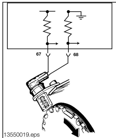
The impulse wheel is mounted behind the crankshaft pulley. The Sensor is mounted on the front timing cover (housing).
