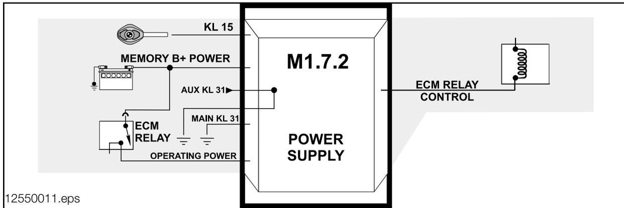
**KL30 - Battery Voltage:** It supplies the operating voltage to the ECM. Battery voltage also sustains system memory for fault codes and adaptation values.
