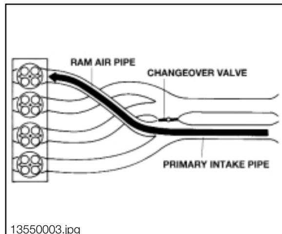
At high rpm, the ECM opens the changeover valve allowing the engine breathing dynamics to change to the dual short air pipes (**volume**). This change enables additional power output at the higher RPM range.
