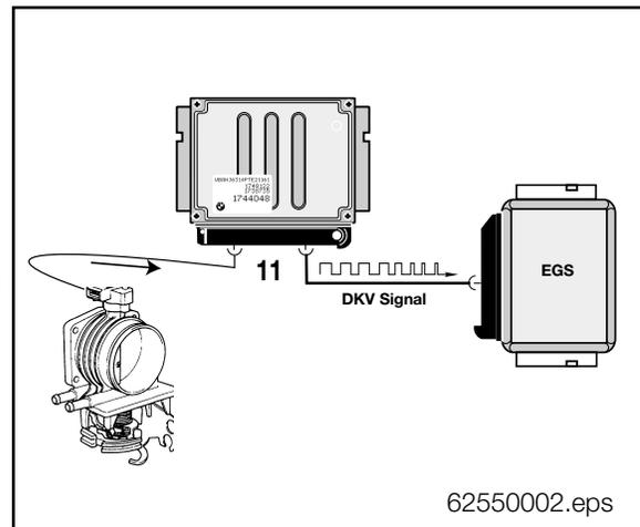
**EGS Ignition Timing Intervention Signal:** The ECM receives an input signal from the EGS Control Module (if equipped) that will retard the ignition timing. This is a momentary ground signal from the EGS during a gear change to reduce engine torque for smoother shifts.
